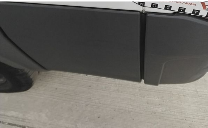
5: Door nsf Scratched Over 25mm Thru Paint
