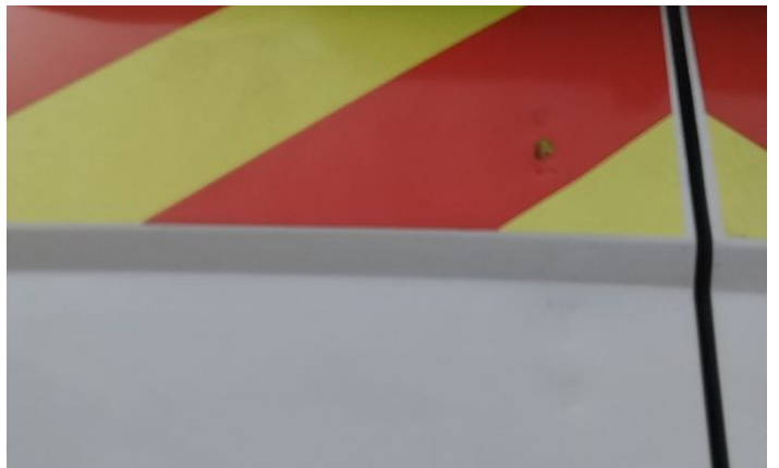
6: Qtr Panel nsr Dented Over 30mm
