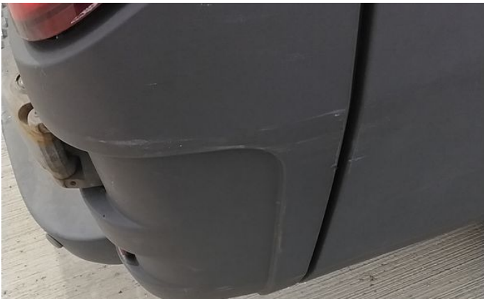
9: Door nsr Dented Over 30mm
