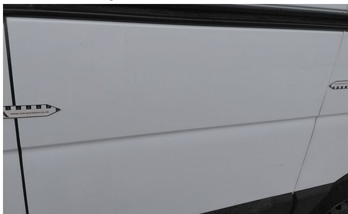
4: Qtr Panel nsr Dented With Paint Damage
