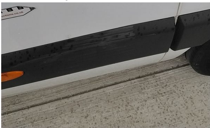
3: Qtr Panel nsr Dented With Paint Damage
