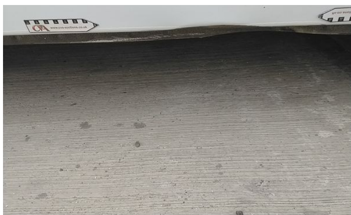
12: Bumper Rear Dented Over 30mm
