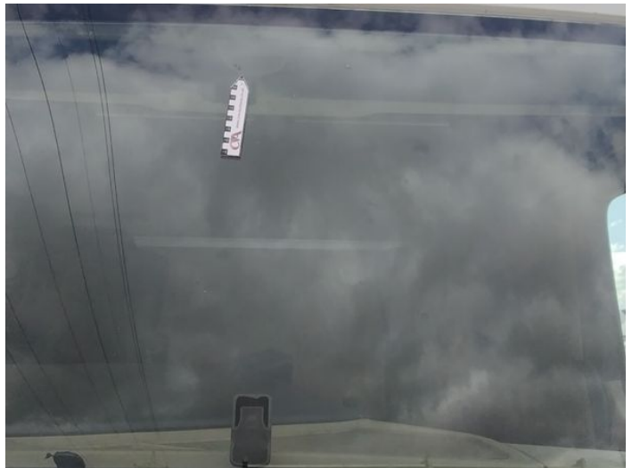
2: Screen Front Chipped Over 10mm
