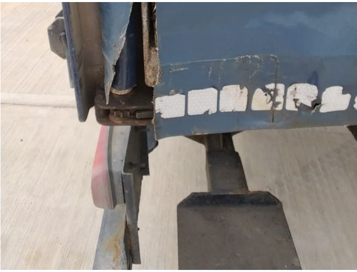
9: Qtr Panel osr Hole Over 10mm
