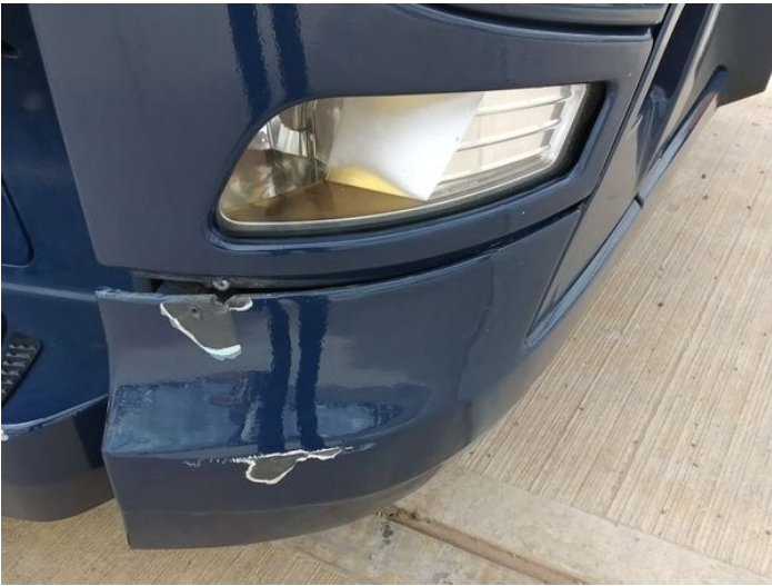
11: Bumper Front Scratched Over 100mm Thru Paint
