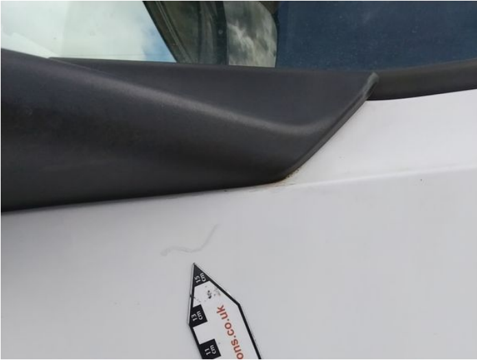
6: Door nsf Scratched Over 25mm Thru Paint
