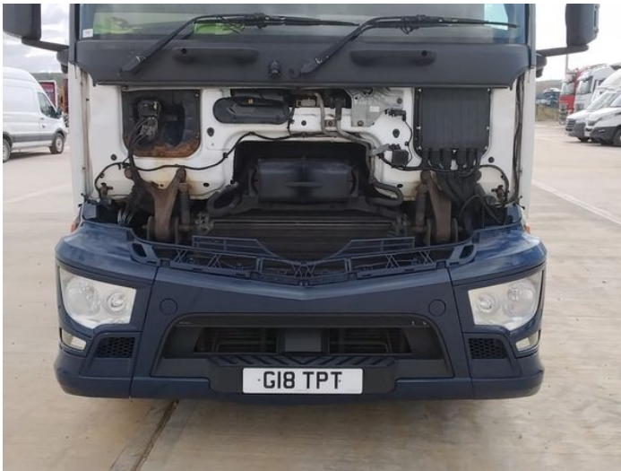
1: Bonnet Missing Replace
