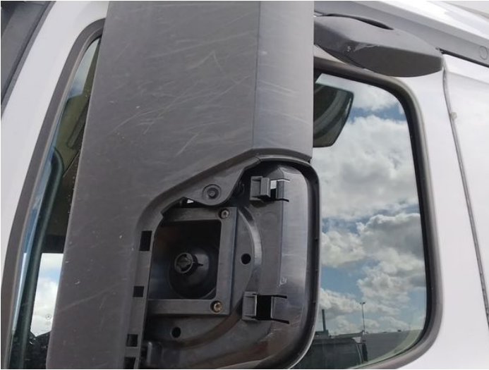
5: Door Mirror Assy nsf Broken Replace
