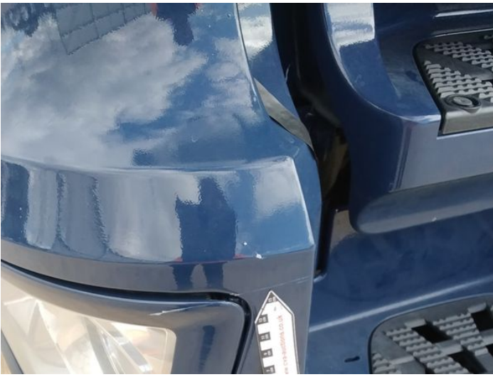
3: Bumper Front Scratched 25 to 100mm Thru Paint
