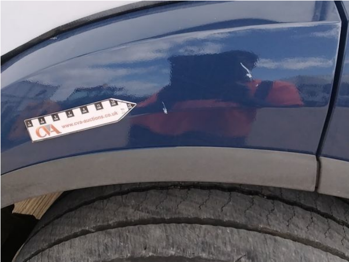
8: Wing Front Arch Extension ns Scratched (Painted) Over 25mm Thru Paint
