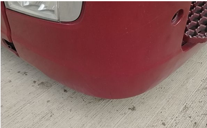
3: Bumper Front Moulding Broken Replace
