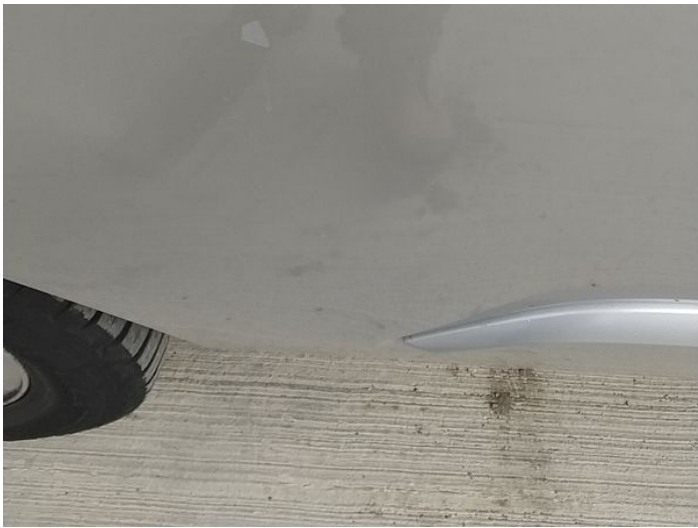
4: Door nsf Chipped Over 5mm
