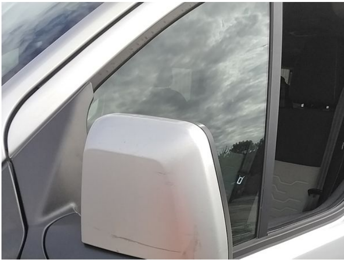
3: Door Mirror Assy nsf Scratched (Painted) Over 25mm Thru Paint
