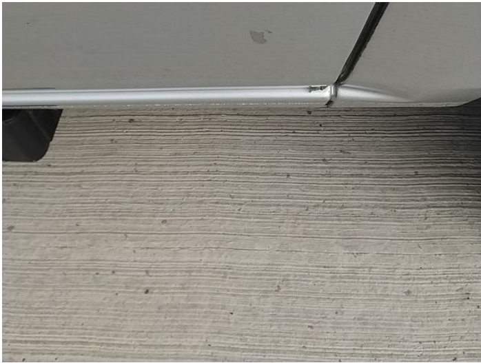
5: Qtr Panel nsr Chipped Over 5mm
