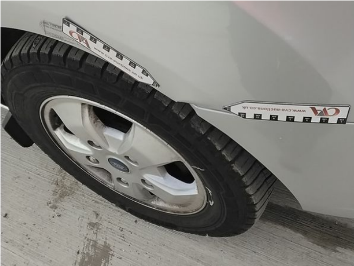
1: Wing osf Dented Over 30mm
