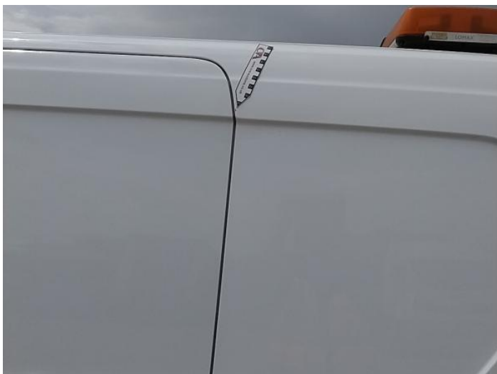
9: Qtr Panel nsr Chipped Over 5mm
