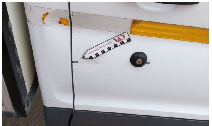
4: Door nsf Rusted Over 5mm
