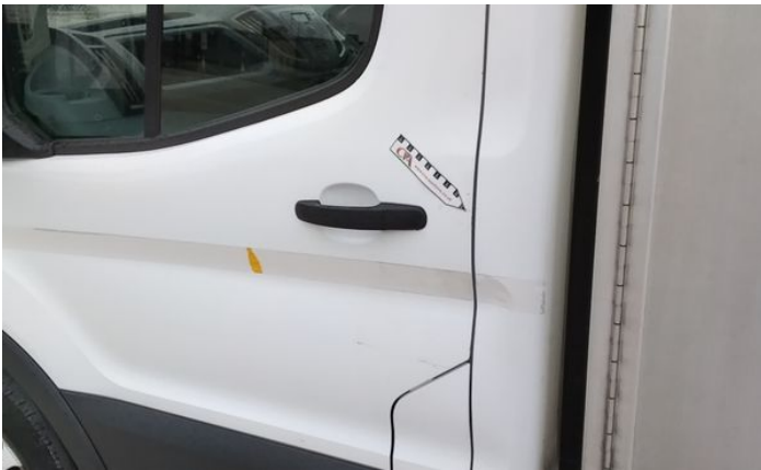
3: A Post ns Scratched UpTo 25mm Not Thru Paint
