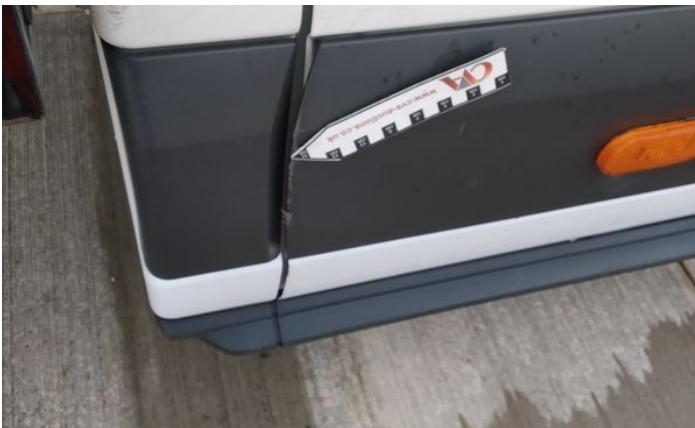
5: Door osf Chipped Multiple Chips
