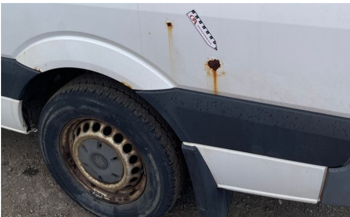
3: Panel Rear Rusted Over 5mm
