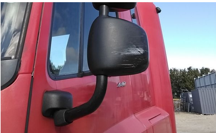
5: Wing nsf Scratched Over 25mm Thru Paint
