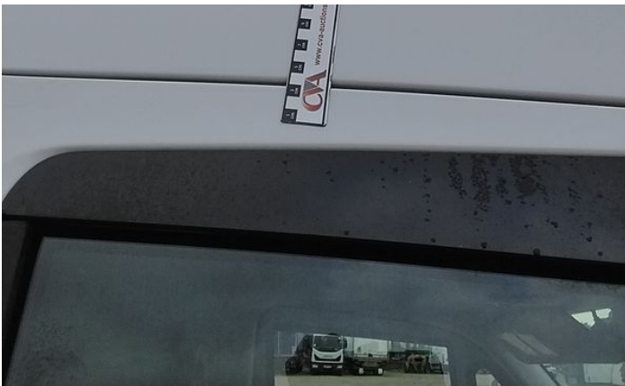
5: Qtr Panel osr Scratched UpTo 25mm Thru Paint
