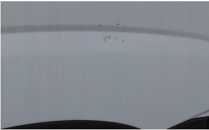
3: Bumper Front Moulding Scuffed (Unpainted) Over 100mm
