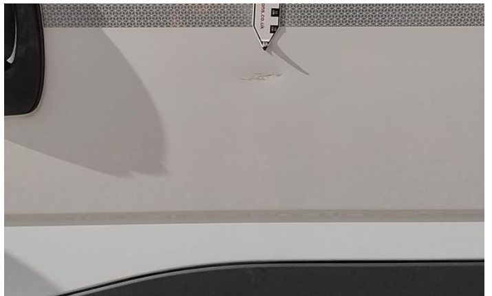
6: Wing nsf Dented Between 10mm + 30mm
