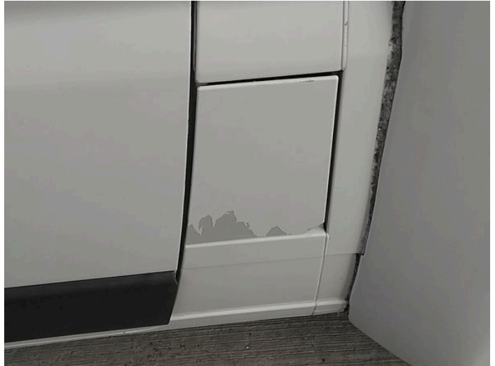
2: Fuel Flap Scratched Over 25mm Thru Paint
