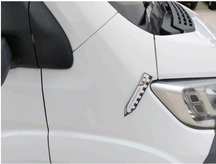
9: Wing osf Chipped Over 5mm
