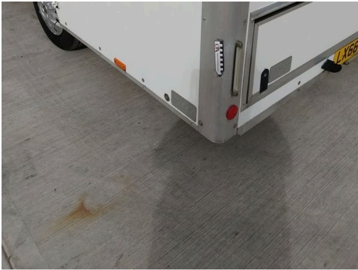
5: Qtr Panel nsr Dented Over 30mm
