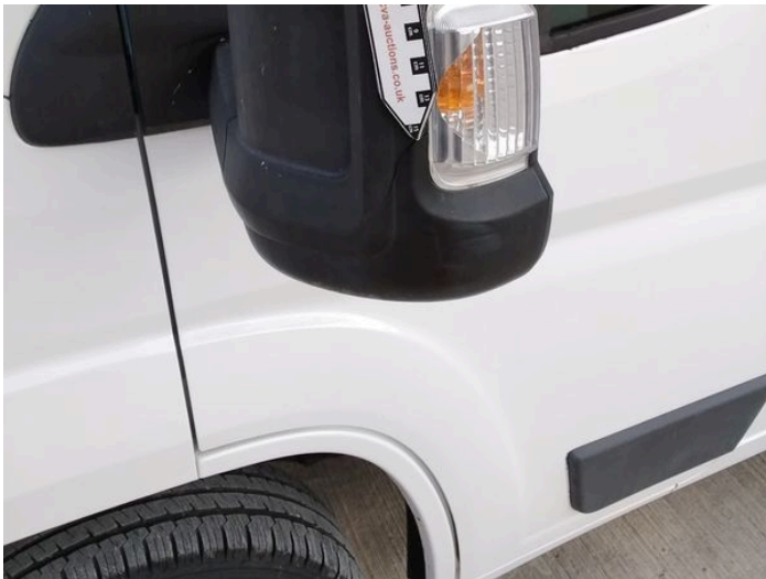
1: Door Mirror Assy nsf Broken Replace
