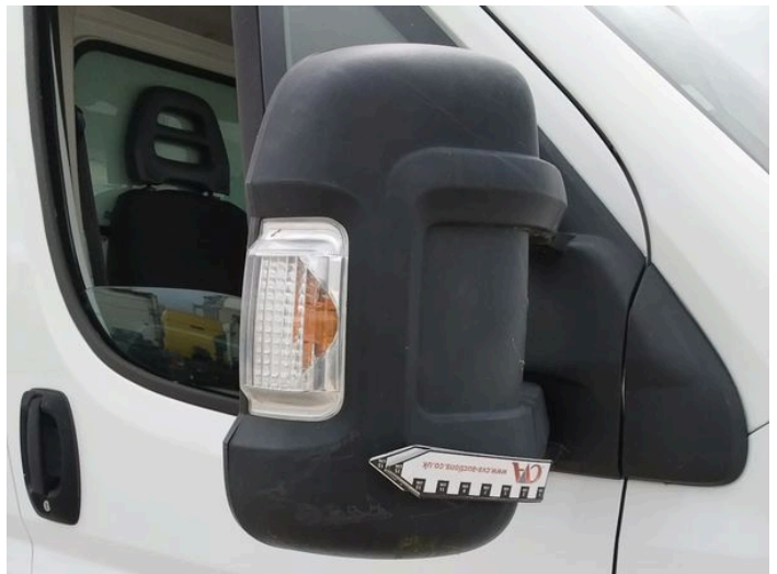
8: Door Mirror Assy osf Scuffed (Unpainted) Over 100mm
