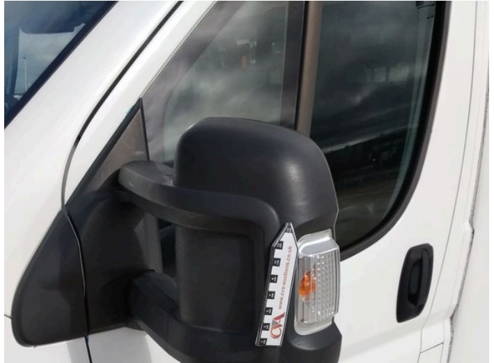
2: Door Mirror Assy nsf Scuffed (Unpainted) Over 100mm
