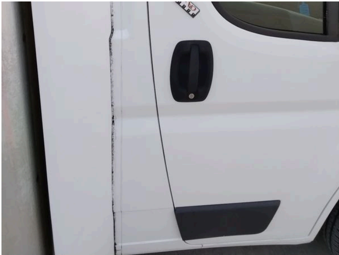
8: Door osf Chipped Over 5mm
