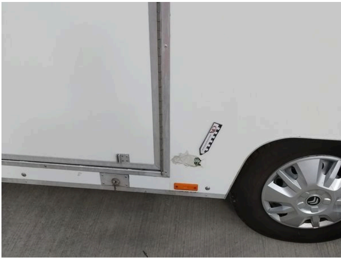
4: Qtr Panel nsr Hole Over 10mm
