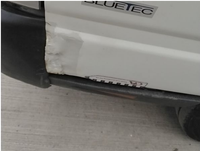
5: Door nsf Dented With Paint Damage
