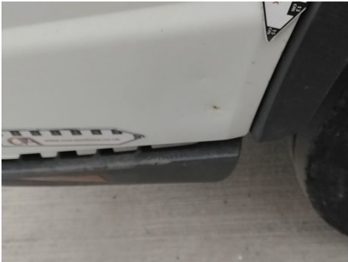
6: Door nsf Dented With Paint Damage
