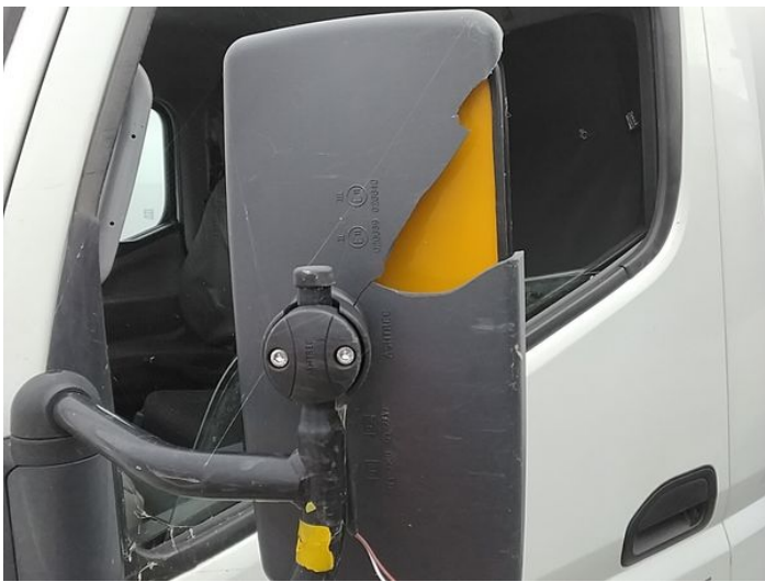
4: Door Mirror Assy nsf Broken Replace
