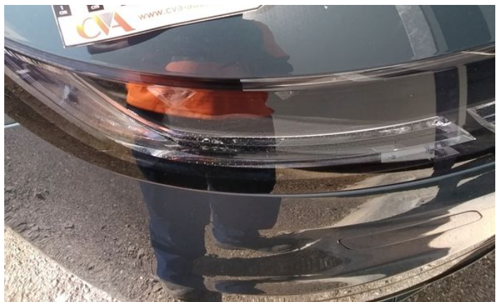
6: Bumper Rear Moulding Scratched (Painted) Over 25mm Thru Paint
