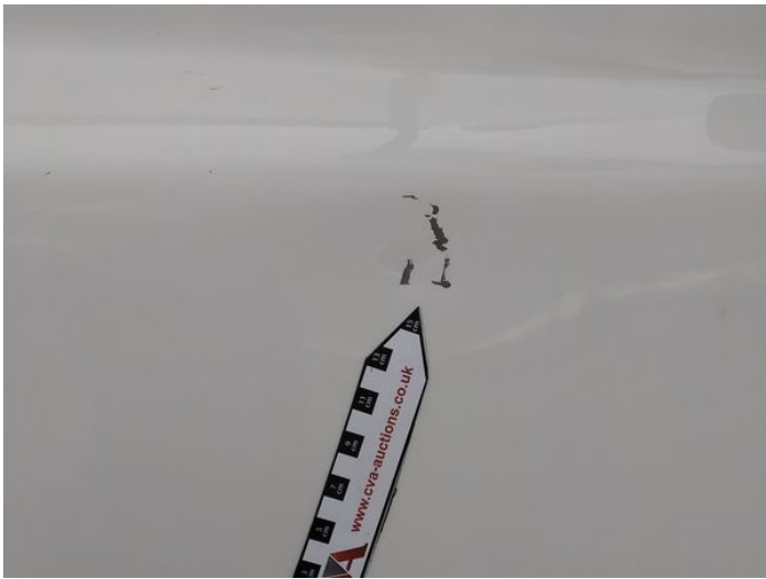
9: Door osf Dented With Paint Damage
