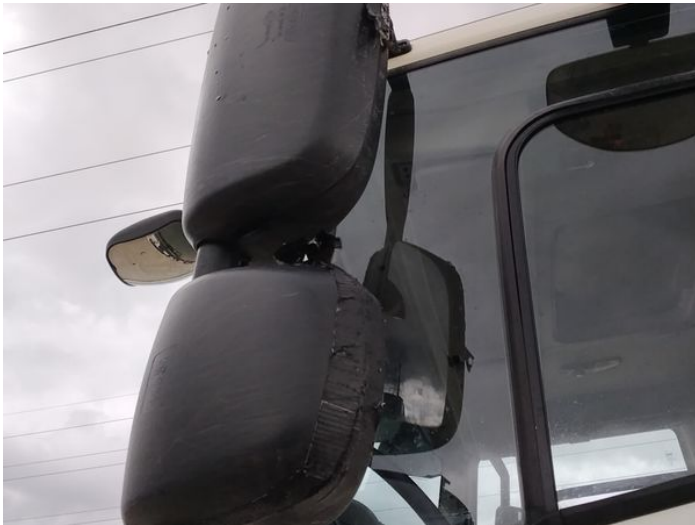
5: Door Mirror Assy nsf Broken Replace
