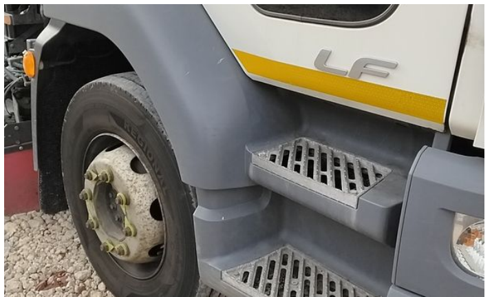
4: Wing Front Arch Extension ns Scuffed (Unpainted) Over 100mm
