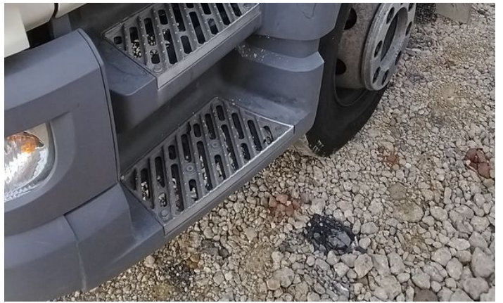
4: Wing nsf Cracked Replace
