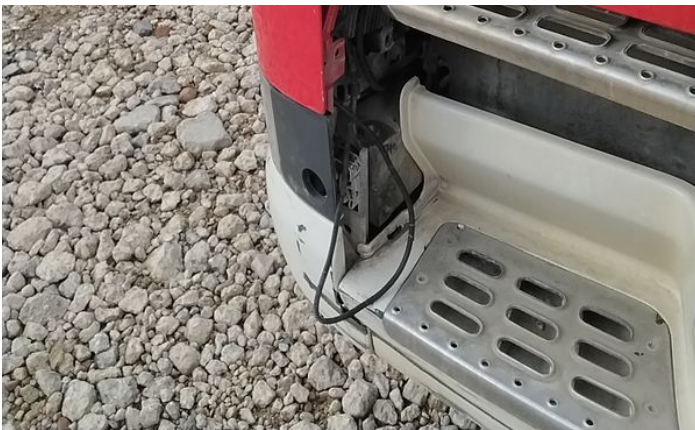
5: Wing Front Arch Extension ns Broken Replace
