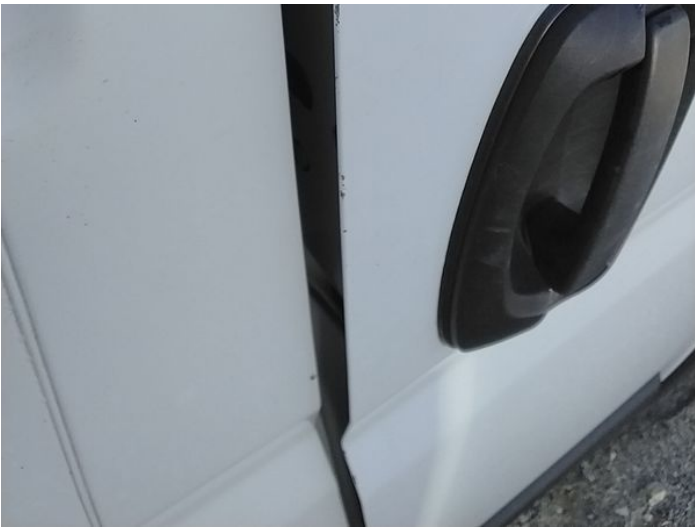
4: Door osf Chipped Edge Chip
