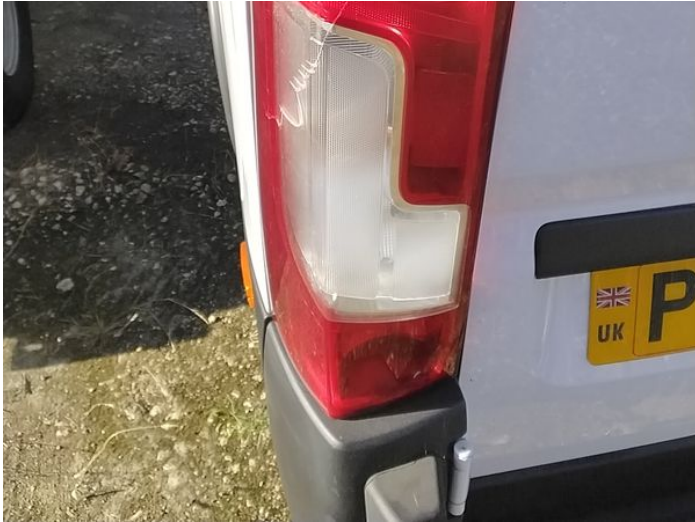
7: Lamp nsr Broken Replace
