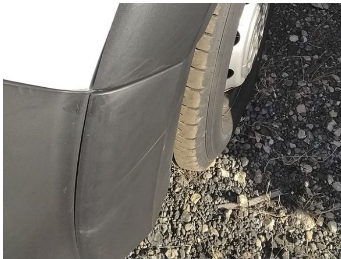
10: Moulding nsf Wing Scuffed (Unpainted) Over 100mm
