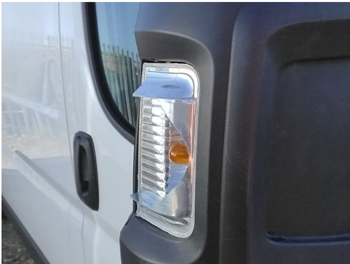
1: Door Mirror Glass os Broken Replace
