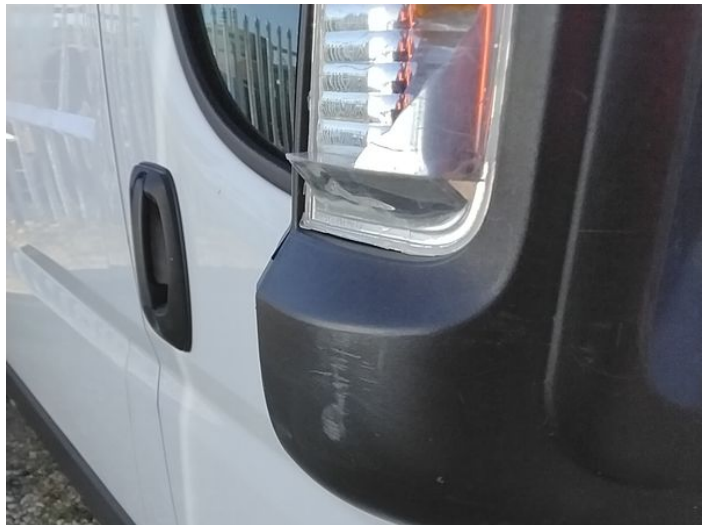
2: Door Mirror Assy osf Scuffed (Unpainted) UpTo 100mm
