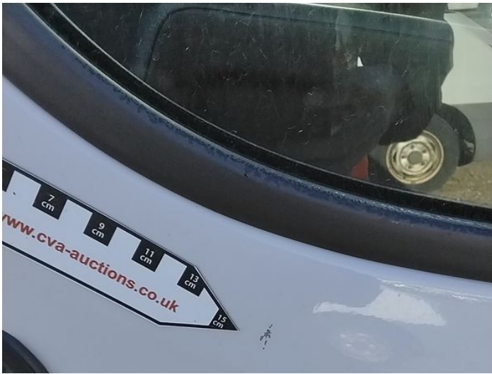
3: Door osf Scratched UpTo 25mm Thru Paint
