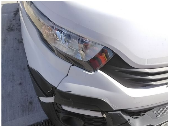
2: Panel Front Cracked Replace
