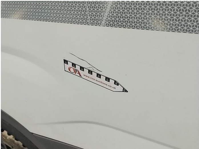
5: Door nsf Scratched Over 25mm Thru Paint
