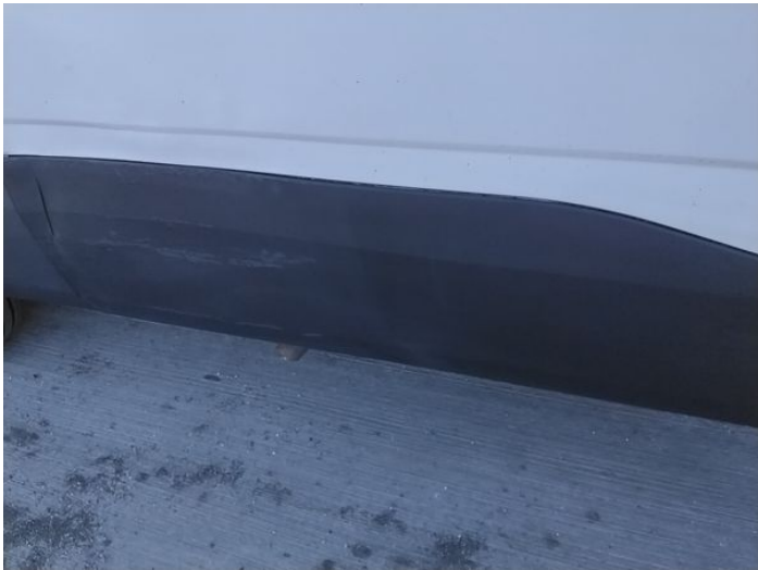
13: Qtr Panel Moulding os Broken Replace
