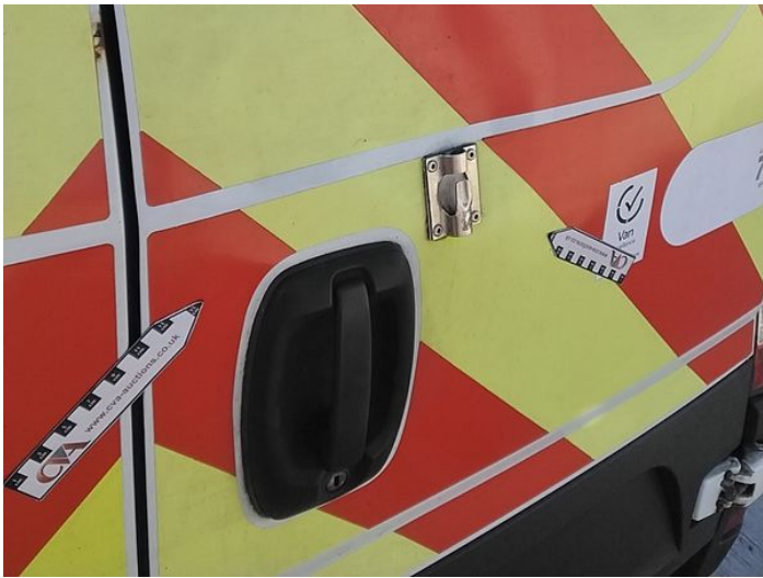
10: Door osr Dented Over 30mm
