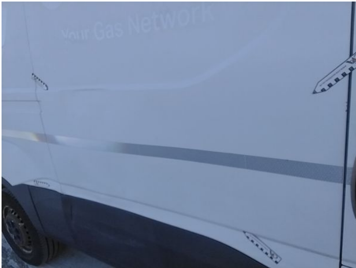
12: Qtr Panel osr Dented Over 30% Of Panel
