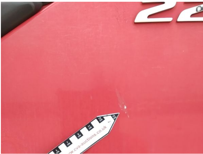
3: Door nsf Scratched Over 25mm Thru Paint
