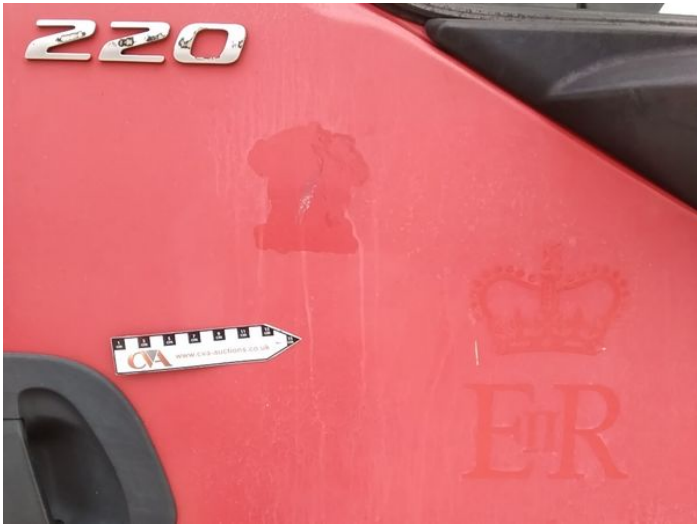
7: Door osf Scratched Over 25mm Thru Paint
