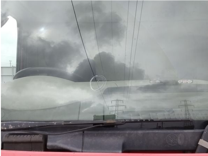
1: Screen Front Cracked Replace
