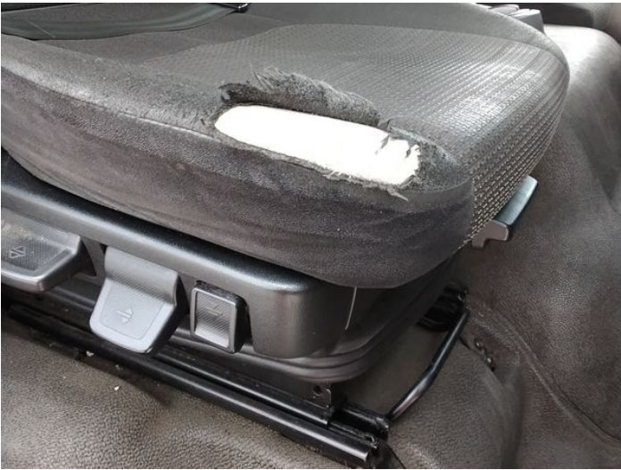
11: Seat Base Cover of Torn Over 3mm
