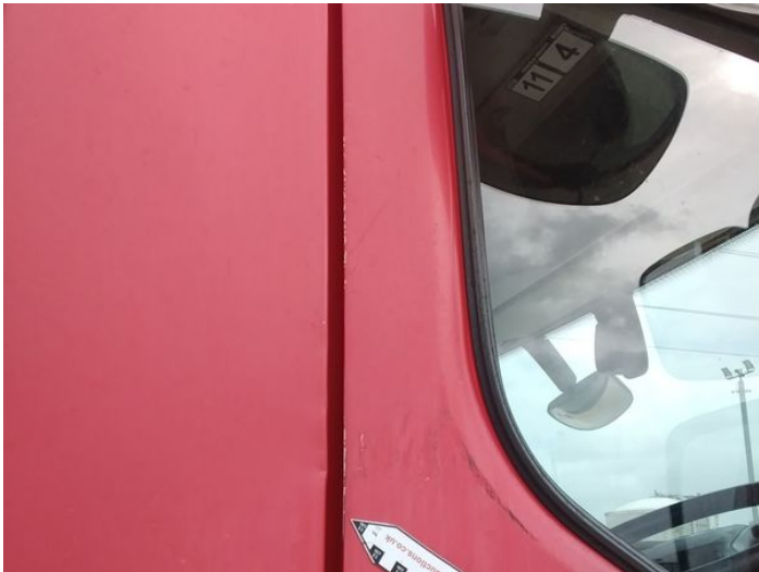
5: Door osf Chipped Multiple Chips
