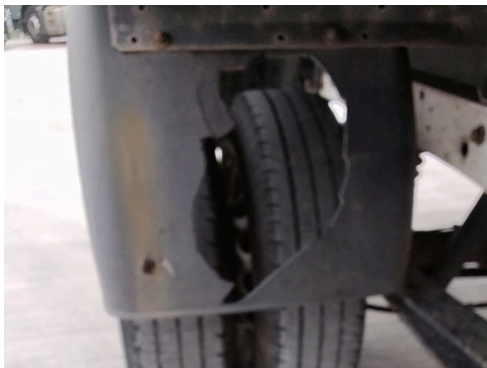
18: Qtr Panel Arch Extension os Broken Replace
