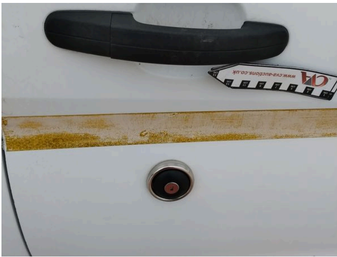
9: Handle Outer osf Scratched (Painted) Over 25mm Not Thru Paint
