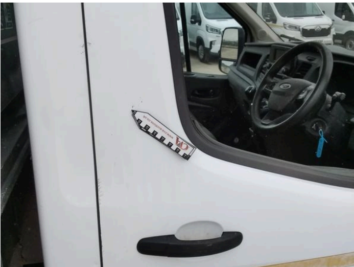
7: Door osf Dented Over 30mm
