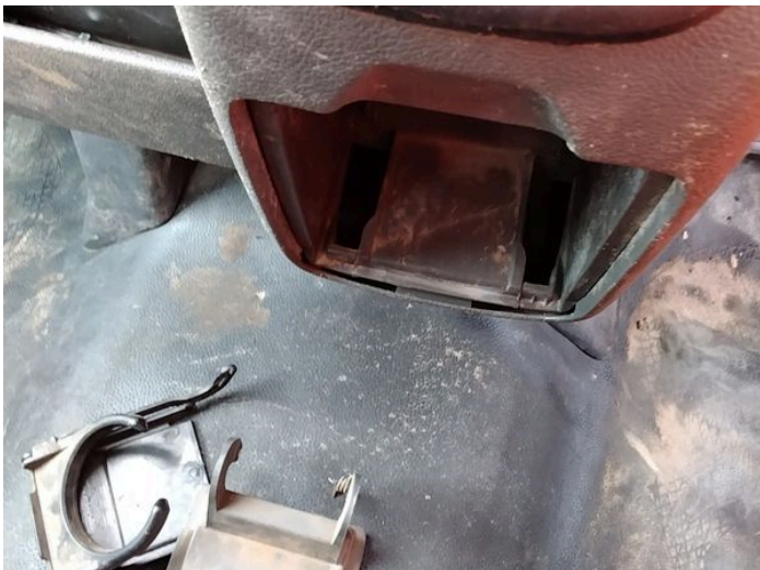
13: Centre Console Front Broken Replace
