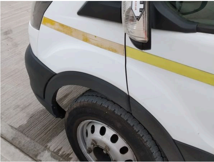
5: Door Mirror Assy nsf Broken Replace
