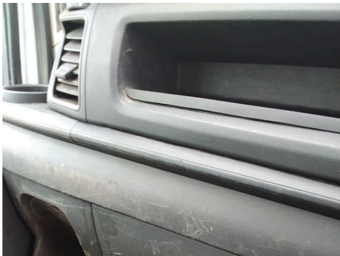
15: Centre Console Front Scuffed Over 25mm
