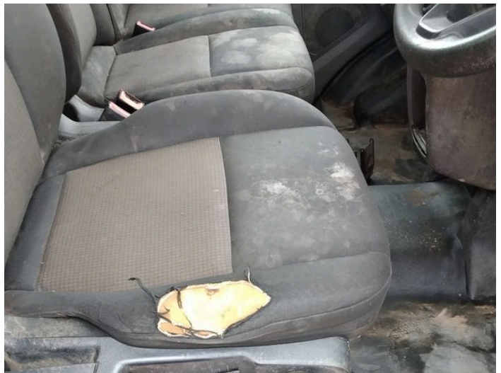
12: Seat Base Cover osf Holed Over 3mm
