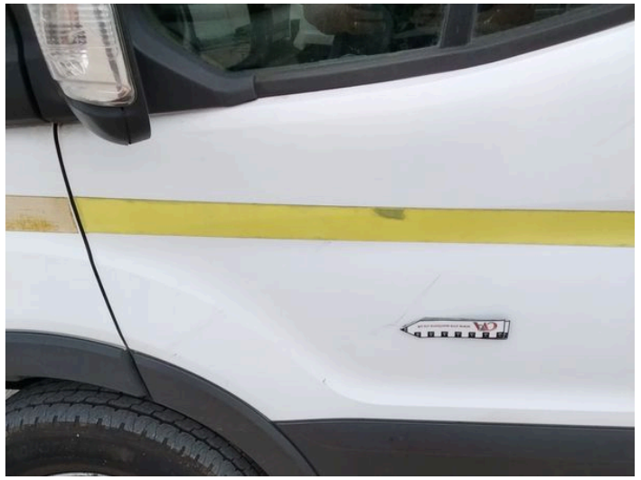
4: Door nsf Scratched Over 25mm Thru Paint
