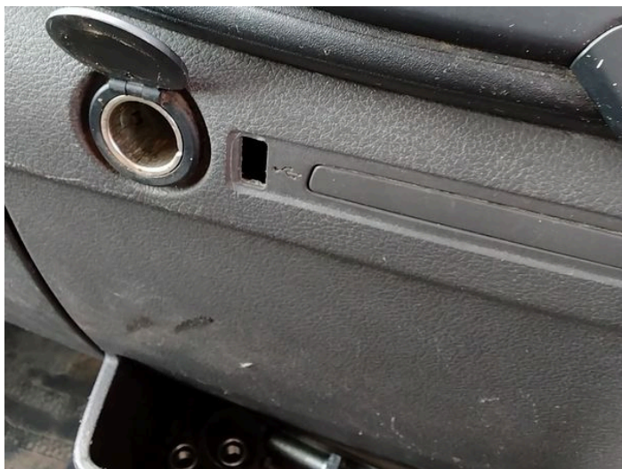
17: Centre Console Front Missing Replace
