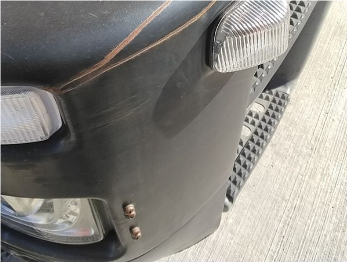
1: Bumper Front Scratched Rusted
