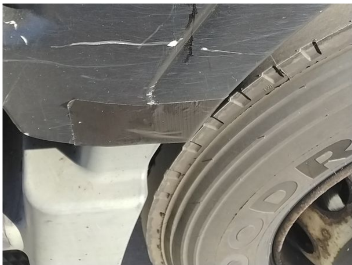
5: Moulding nsf Wing Broken Replace
