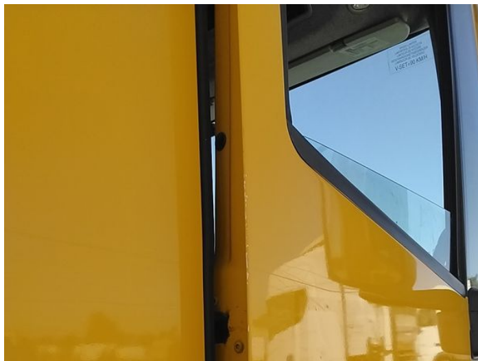
4: Door osf Chipped Edge Chip
