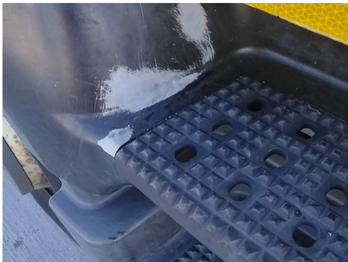
3: Qtr Panel Arch Extension os Scratched (Painted) Over 25mm Thru Paint
