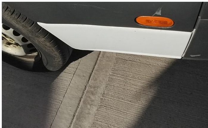
4: Qtr Panel nsr Dented Over 30mm
