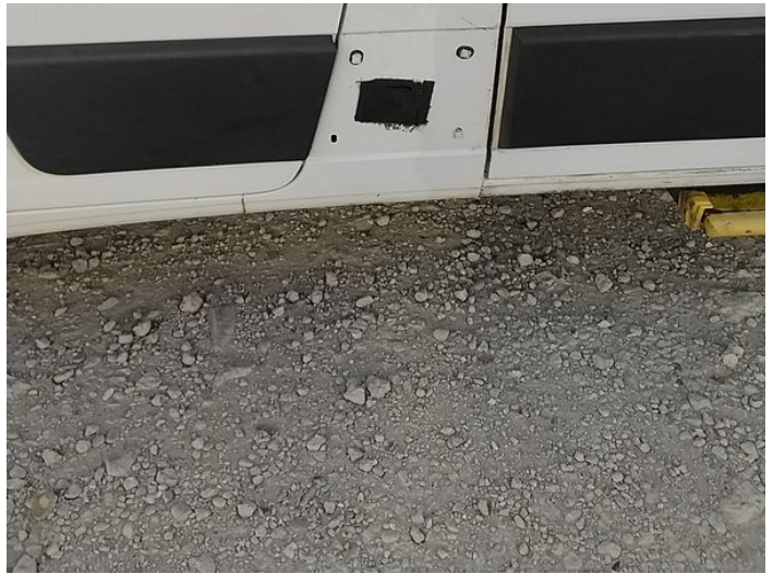
6: Qtr Panel Moulding ns Missing Replace
