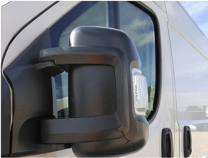
5: Door Mirror Assy nsf Broken Replace
