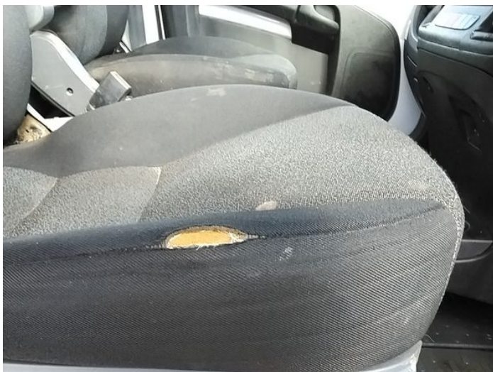
14: Seat Base Cover osf Holed Over 3mm
