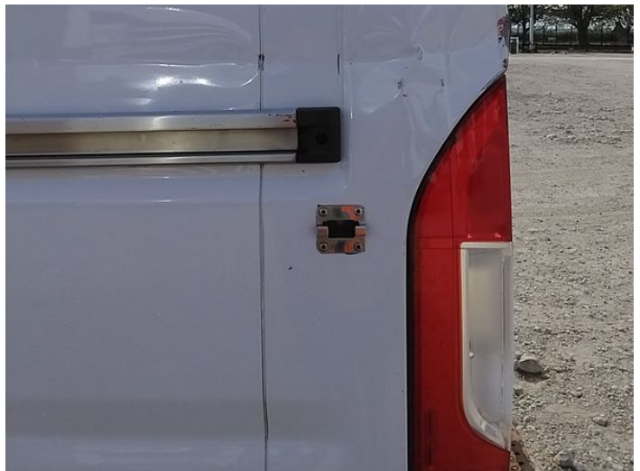
8: Qtr Panel nsr Dented With Paint Damage
