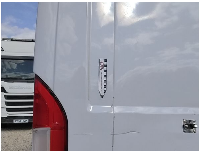
10: Qtr Panel osr Scratched Over 25mm Thru Paint
