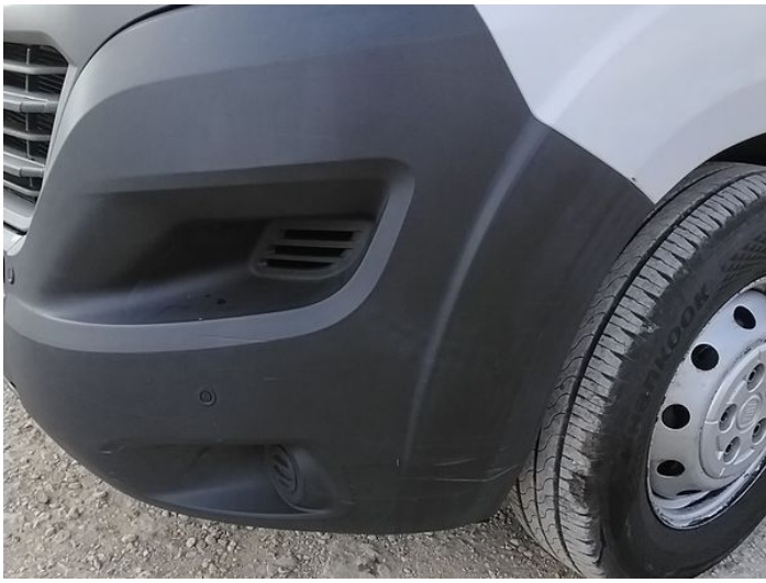
3: Bumper Front Moulding Scuffed (Unpainted) UpTo 100mm
