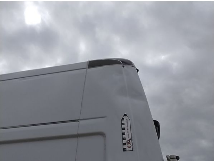
7: Qtr Panel nsr Dented Over 30mm
