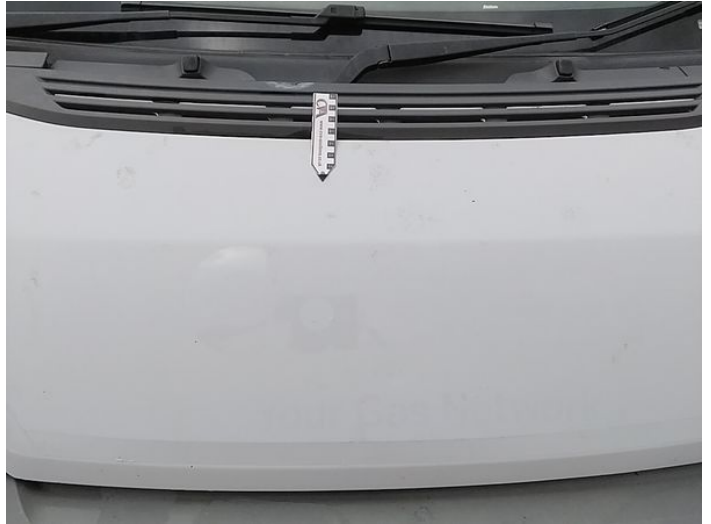
2: Bonnet Scratched Over 25mm Thru Paint
