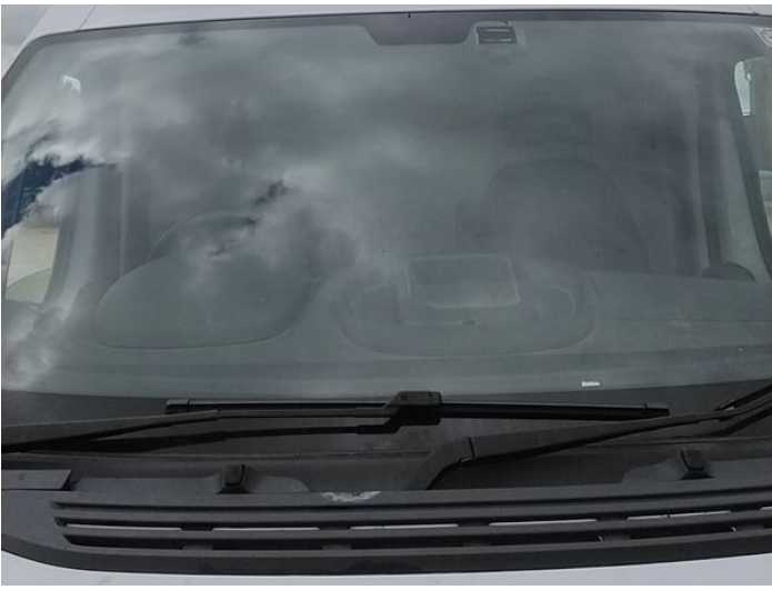
3: Screen Front Chipped Over 10mm
