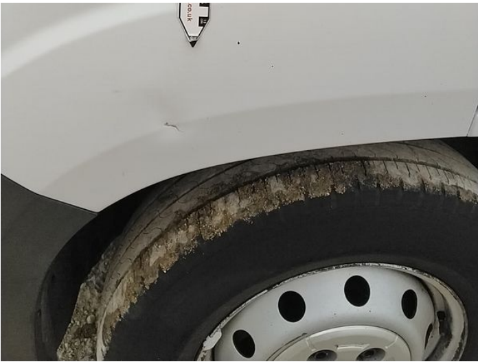
4: Wing nsf Scratched UpTo 25mm Thru Paint
