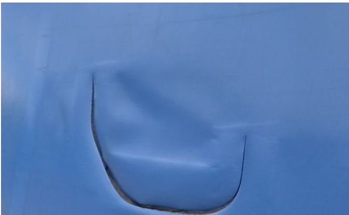
11: Qtr Panel nsr Dented Over 30mm
