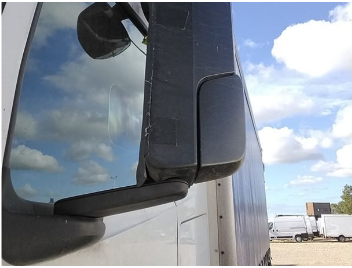
3: Door Mirror Assy nsf Broken Replace
