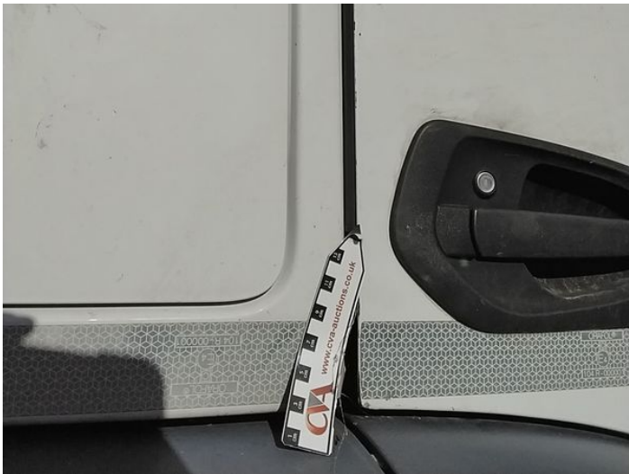
10: Door osf Chipped Edge Chip
