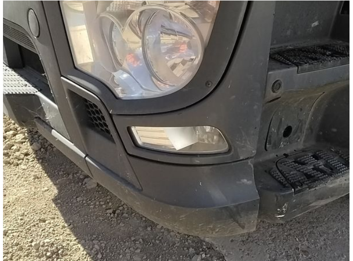
2: Bumper Front Moulding Scuffed (Unpainted) UpTo 100mm
