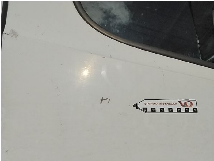
9: Door osf Scratched UpTo 25mm Thru Paint
