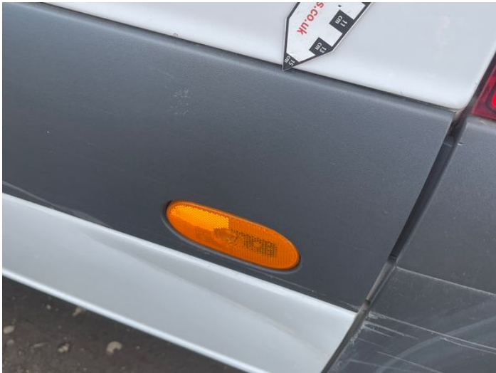
13: Qtr Panel nsr Dented With Paint Damage
