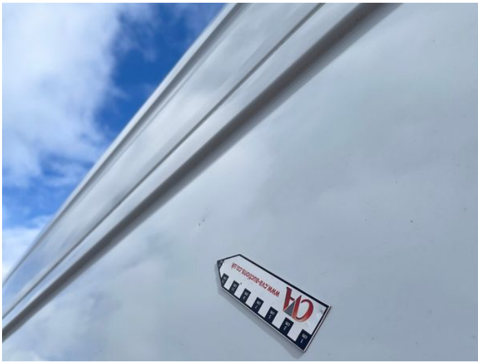
9: Qtr Panel osr Dented Over 30mm
