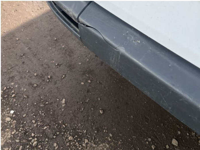
11: Bumper Rear Moulding Broken Replace
