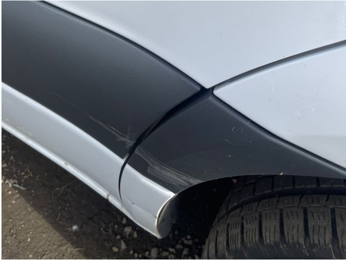
6: Door Moulding osf Scuffed (Unpainted) Over 100mm
