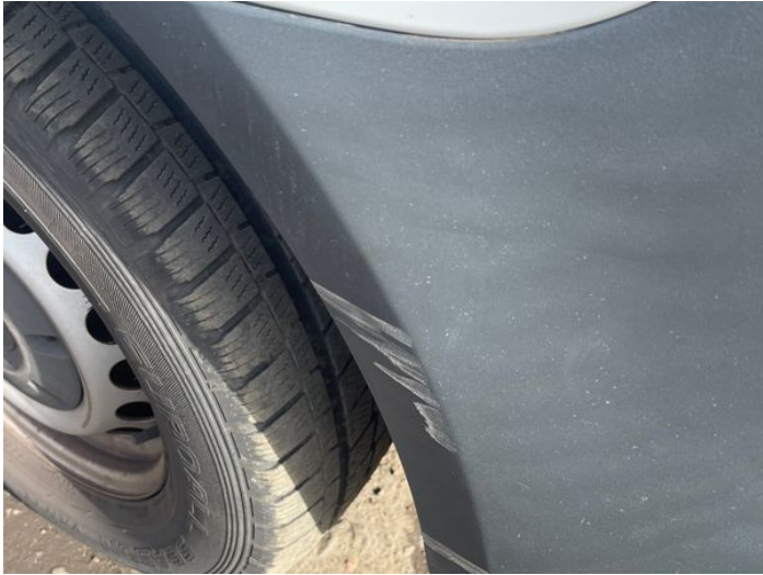
5: Bumper Front Moulding Scuffed (Unpainted) Over 100mm
