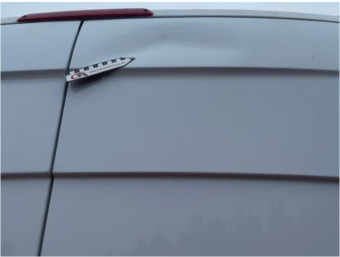
4: Tailgate Dented With Paint Damage
