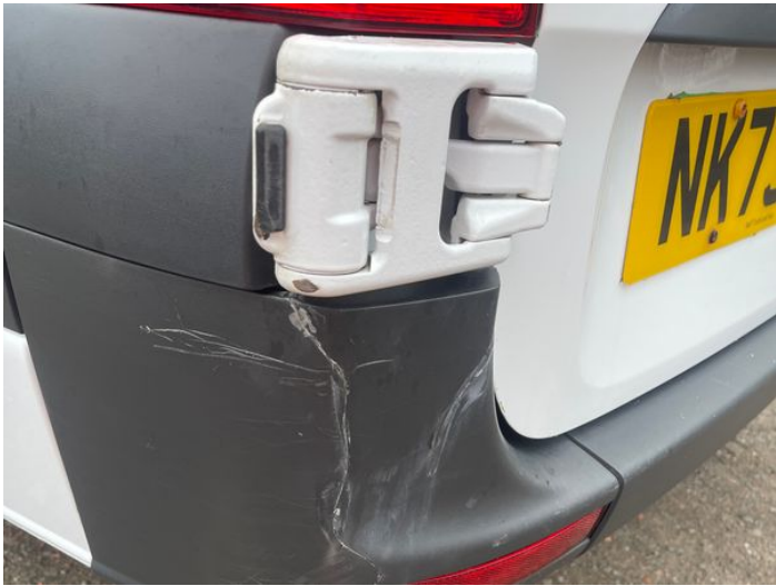
5: Qtr Panel nsr Cracked Replace
