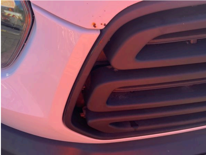
1: Bonnet Rusted Over 5mm
