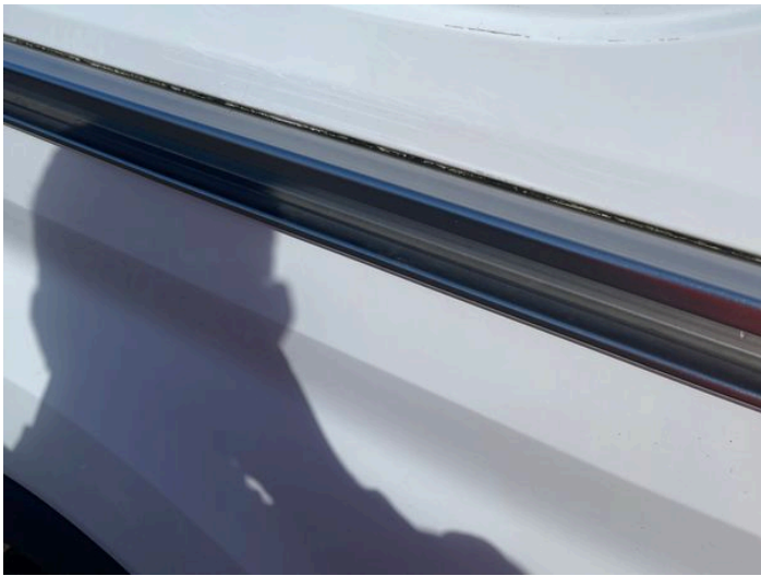
3: Panel Rear Scratched Over 25mm Thru Paint
