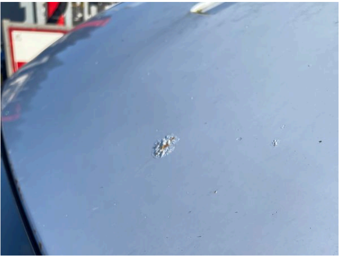
4: Roof Rusted Over 5mm
