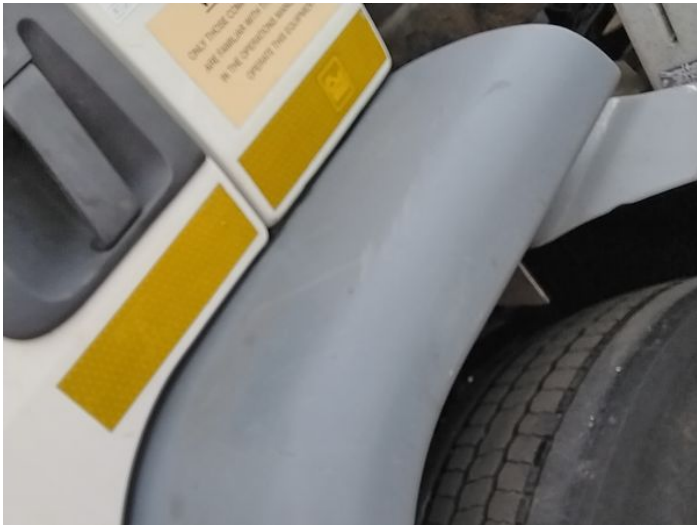
11: Wing nsf Scratched Over 25mm Thru Paint
