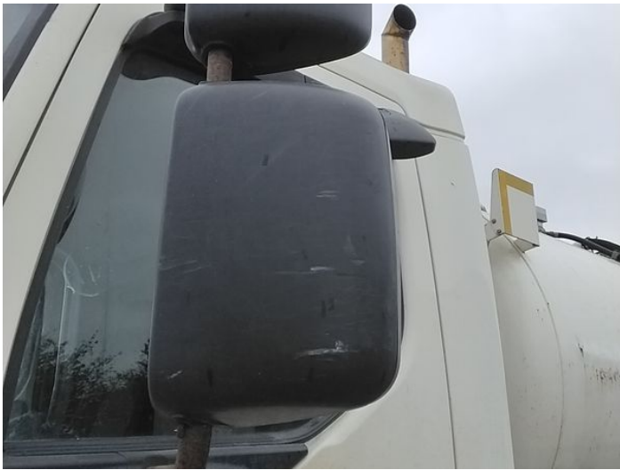
9: Door Mirror Assy nsf Scuffed (Unpainted) Over 100mm
