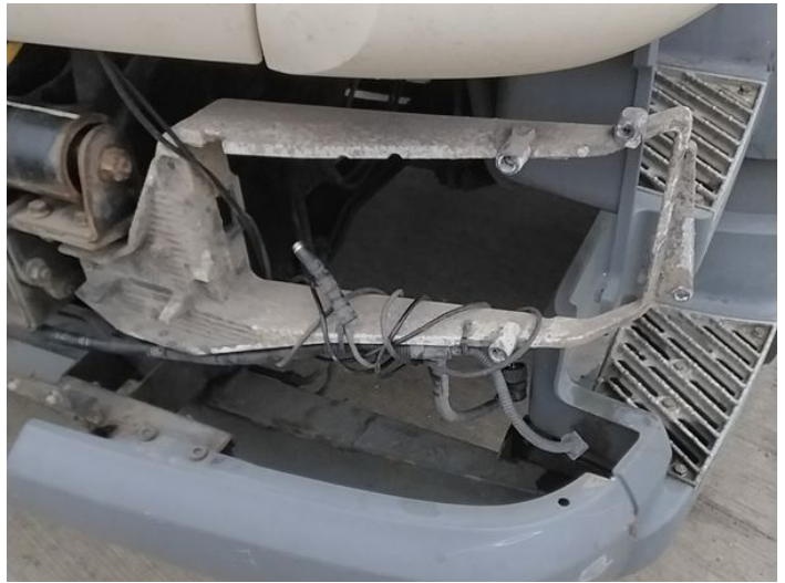
6: Headlamp ns Missing Replace
