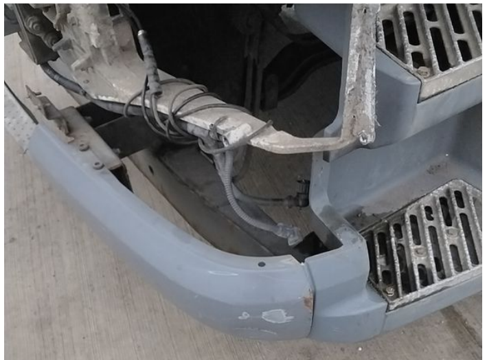
8: Bumper Front Dented With Paint Damage
