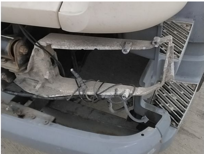
7: Panel Front Missing Replace
