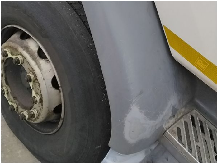
12: Wing osf Scratched Over 25mm Thru Paint
