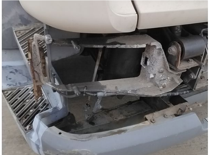
2: Headlamp os Missing Replace
