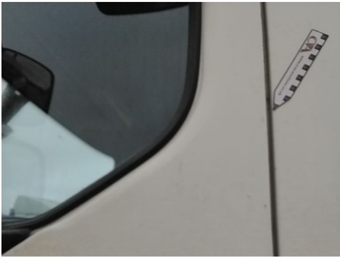
10: Door nsf Scratched Over 25mm Thru Paint
