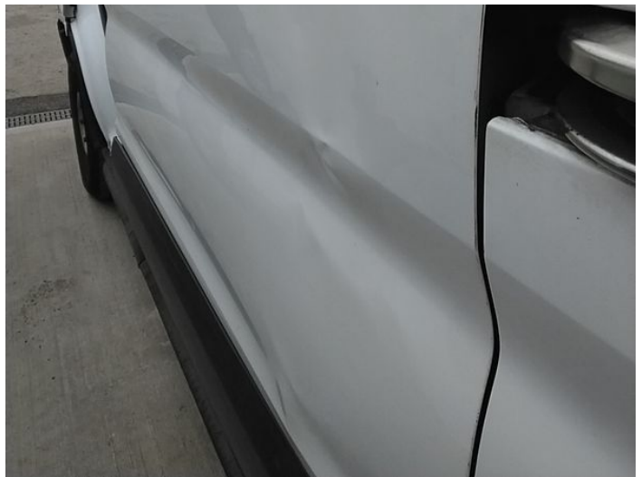
18: Door nsr Dented Over 30% Of Panel
