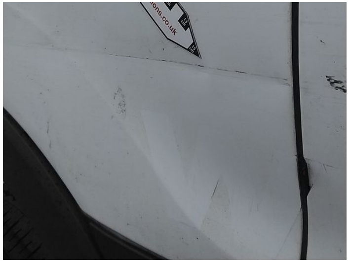
10: Qtr Panel osr Dented Over 30mm
