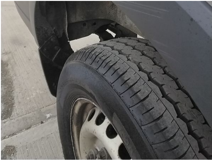
11: Qtr Panel Trim os Scuffed Over 25mm
