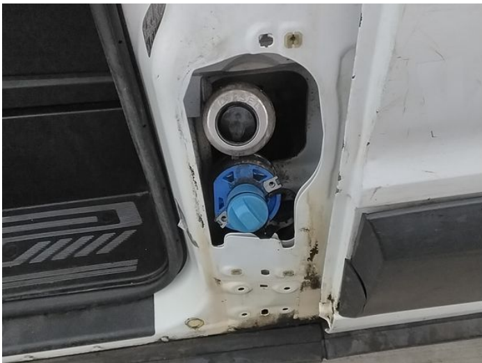
19: Fuel Flap Missing Replace
