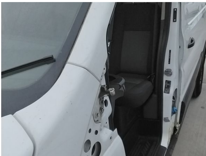
6: Door Mirror Assy nsf Missing Replace
