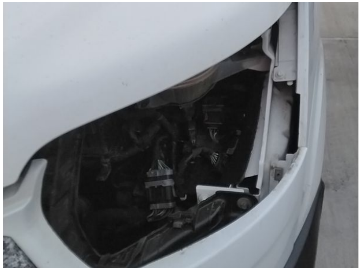
2: Headlamp ns Missing Replace
