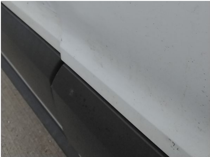
13: Door osf Dented Over 30mm
