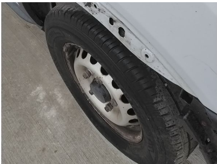
8: Moulding osf Wing Broken Replace
