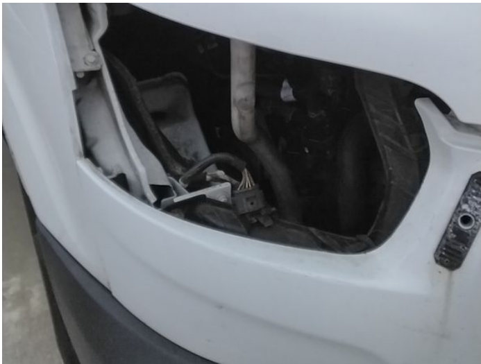
1: Headlamp os Missing Replace
