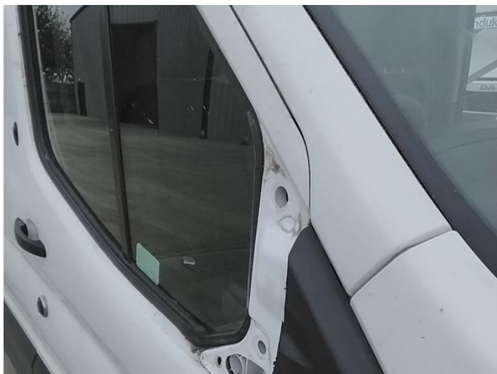
5: Door Mirror Assy osf Missing Replace
