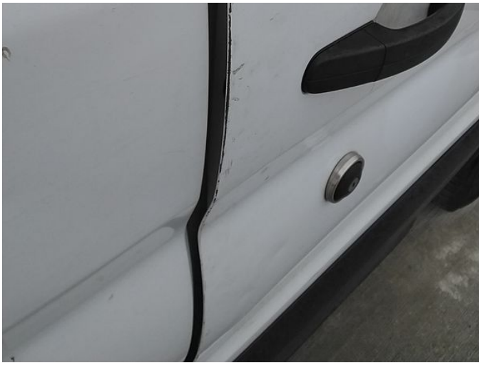
9: Door osf Chipped Edge Chip
