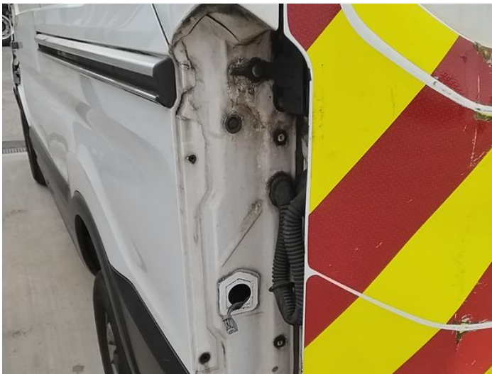
17: Lamp nsr Missing Replace
