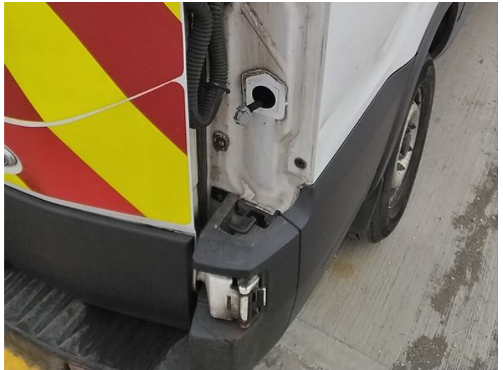
14: Lamp osr Missing Replace
