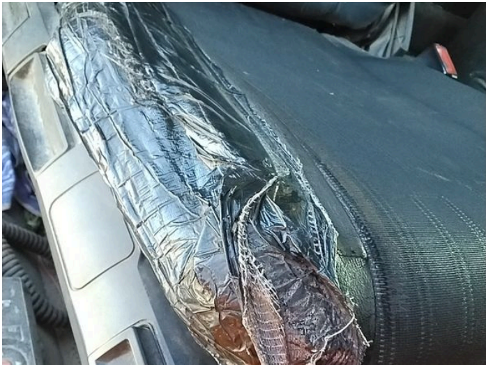
14: Seat Base Cover osf Torn Over 3mm
