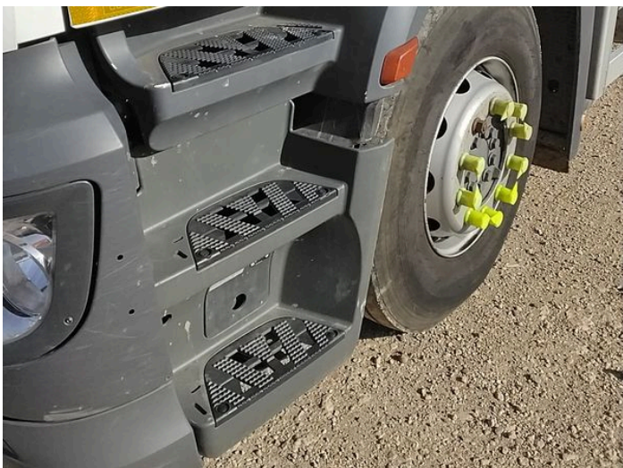
7: Wing Front Arch Extension nsf Scuffed (Unpainted) Over 100mm
