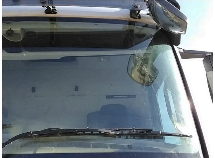
2: Screen Front Chipped Over 10mm
