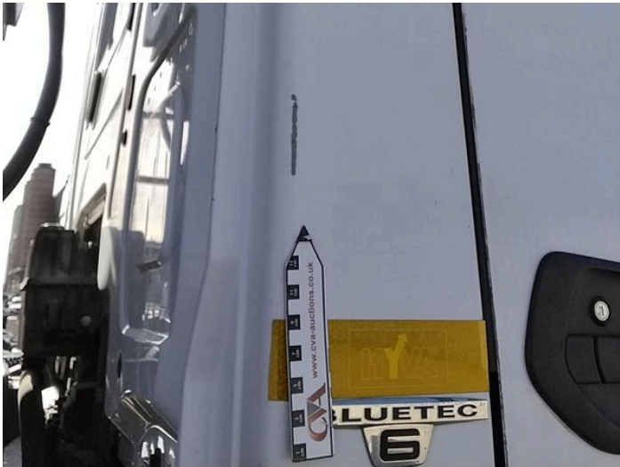
12: B Post os Scratched UpTo 25mm Thru Paint
