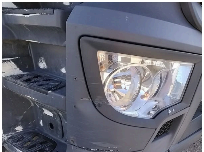
4: Bumper Front Dented With Paint Damage
