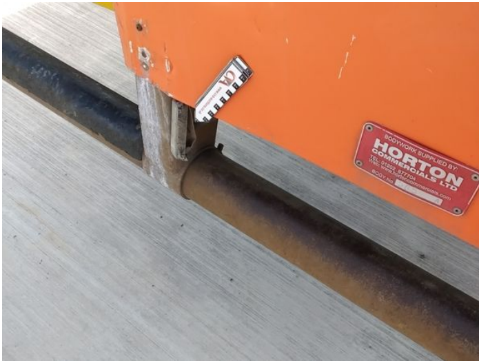
19: Reflector nsr Broken Replace
