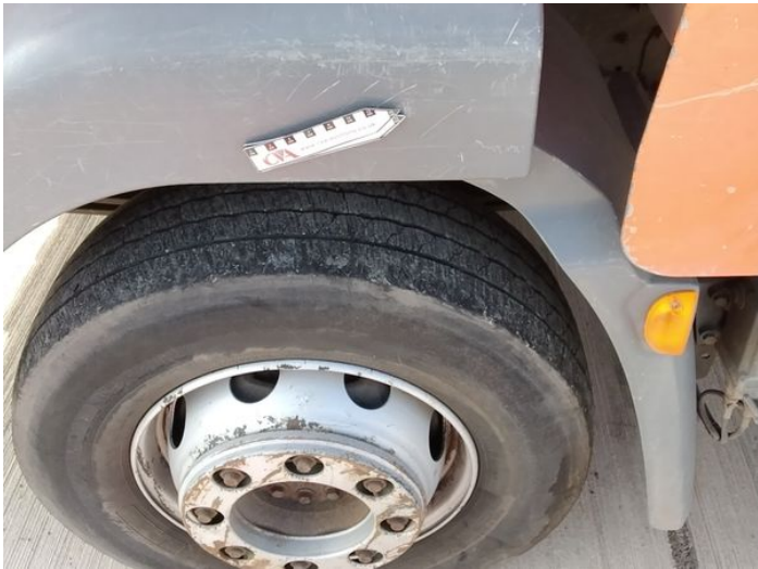
8: Qtr Panel Arch Extension ns Scuffed (Unpainted) Over 100mm
