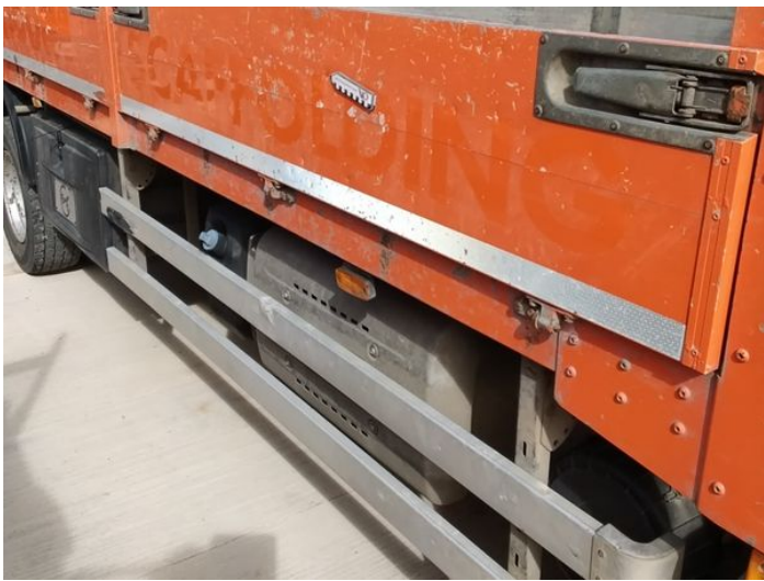
27: Qtr Panel osr Dented Over 30mm
