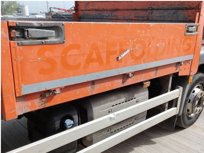
26: Qtr Panel osr Chipped Over 5mm
