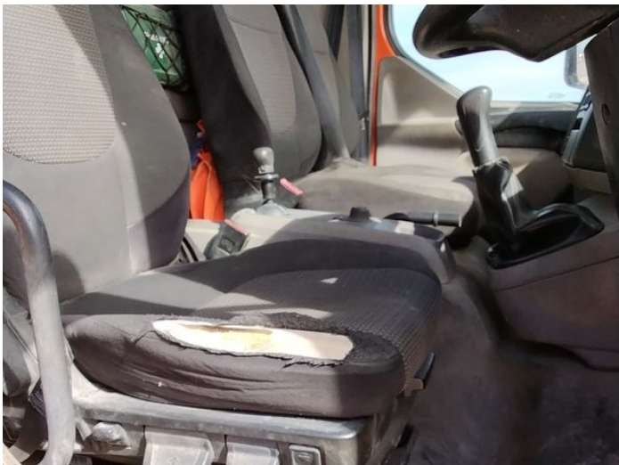
37: Seat Base Cover osf Torn Over 3mm
