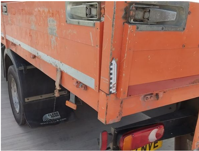
15: Qtr Panel nsr Chipped Over 5mm
