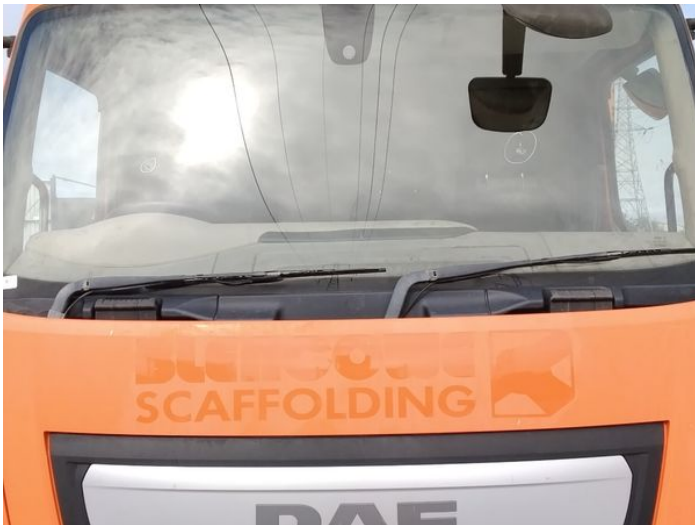
1: Screen Front Chipped Over 10mm
