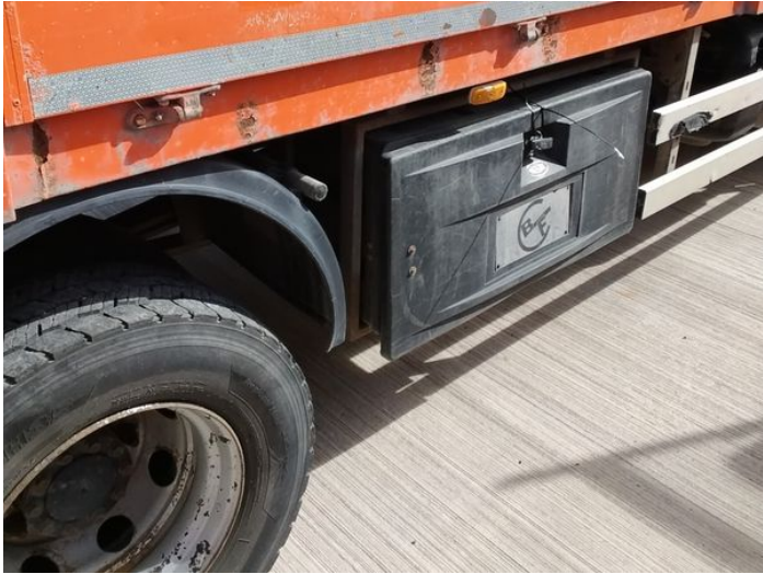
23: Qtr Panel osr Chipped Over 5mm
