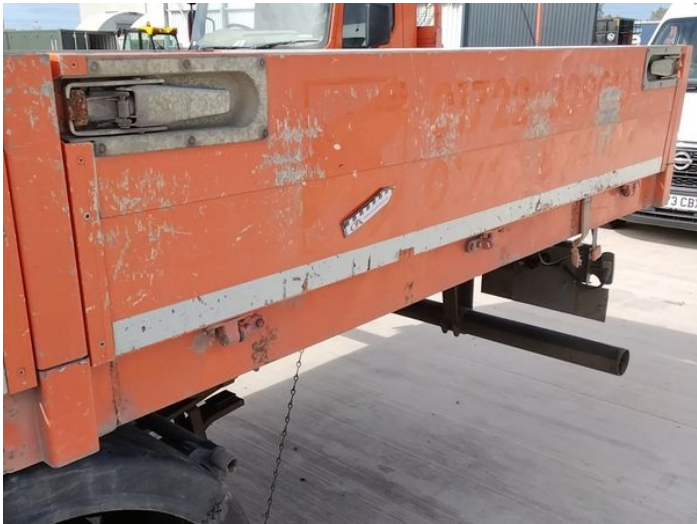
13: Qtr Panel nsr Chipped Over 5mm
