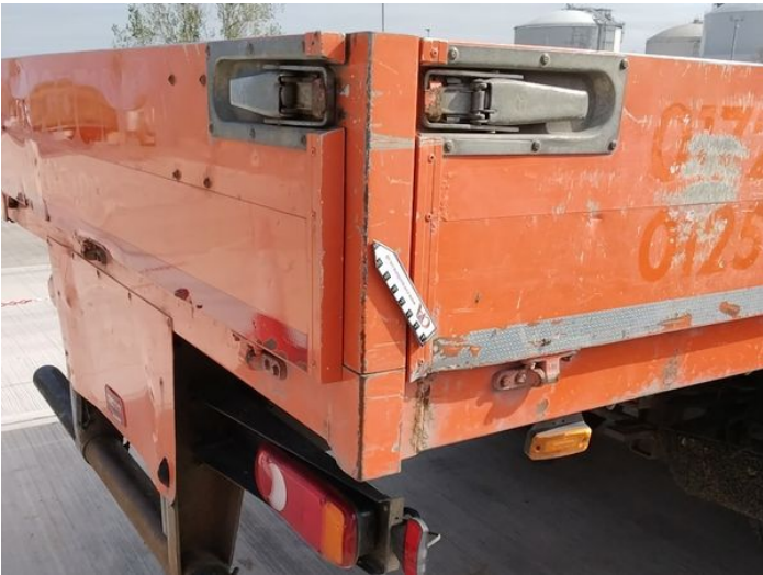
20: Qtr Panel osr Chipped Multiple Chips
