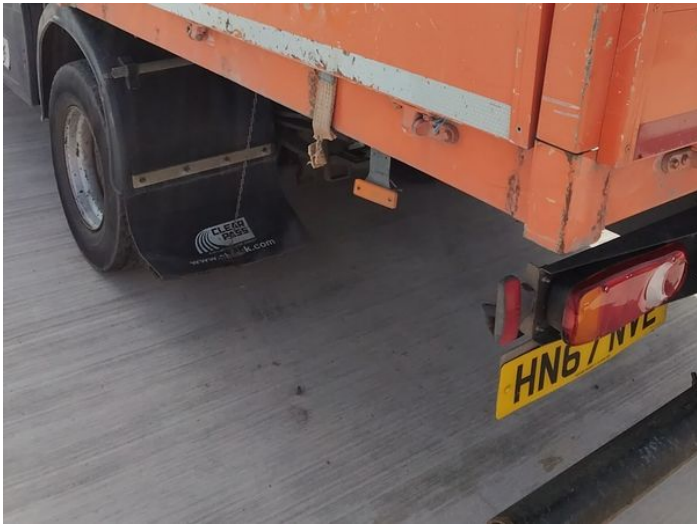
14: Qtr Panel nsr Dented Over 30mm
