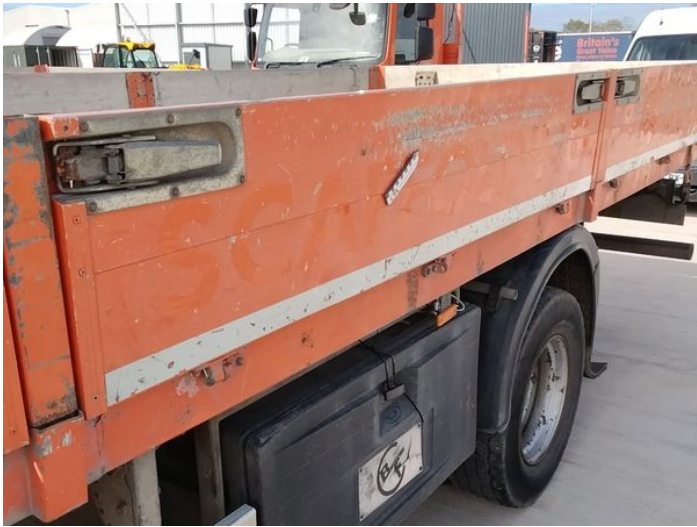
11: Qtr Panel nsr Chipped Over 5mm
