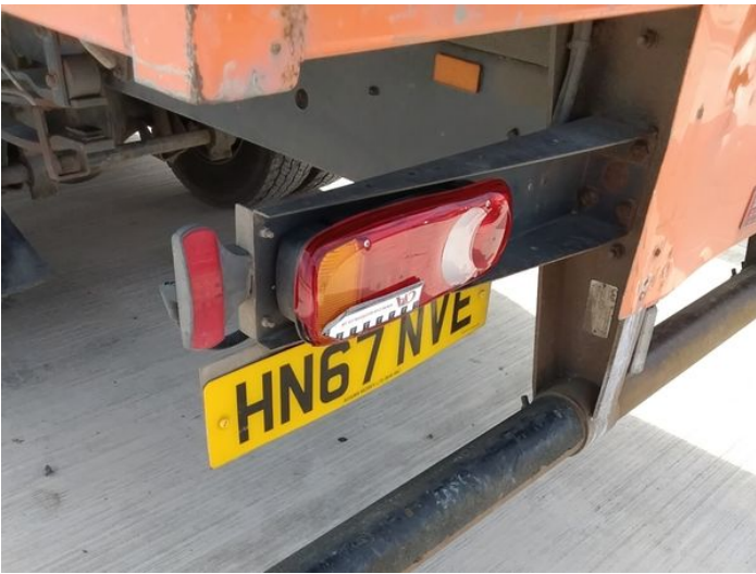
16: Lamp nsr Broken Replace
