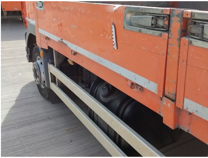
10: Qtr Panel nsr Dented Over 30mm
