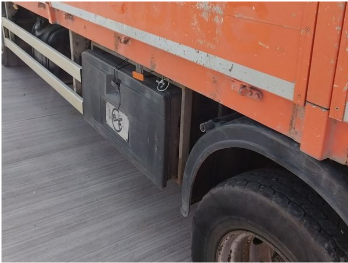
12: Qtr Panel nsr Dented Over 30mm
