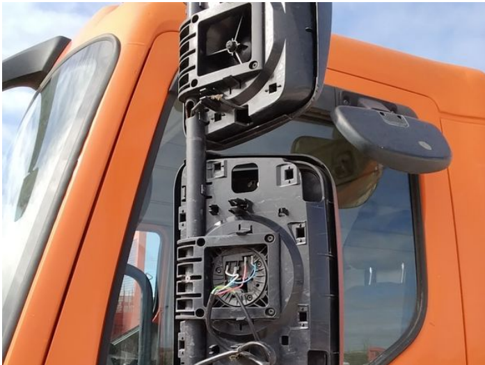
5: Door Mirror Assy nsf Missing Replace
