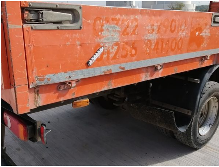
21: Qtr Panel osr Chipped Over 5mm
