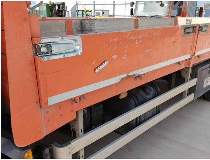
9: Qtr Panel nsr Chipped Over 5mm
