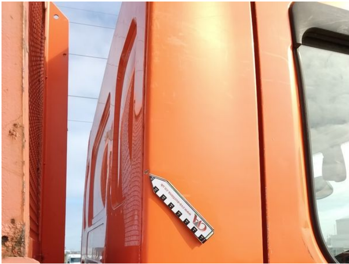
29: Panel Rear Chipped Over 5mm
