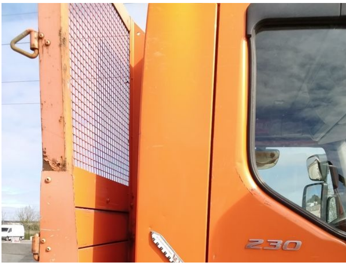
28: Panel Rear Dented Over 30mm
