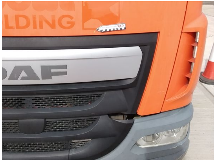
2: Bonnet Chipped Over 5mm
