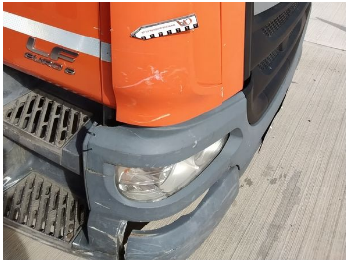
34: Moulding osf Wing Scratched (Painted) Over 25mm Thru Paint
