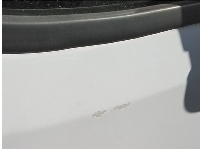
2: Door osf Chipped Over 5mm
