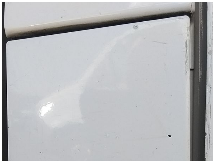
4: Fuel Flap Scratched Over 25mm Not Thru Paint
