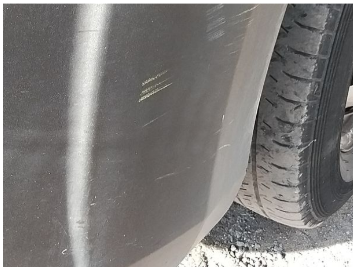
6: Bumper Front Moulding Scuffed (Unpainted) Over 100mm
