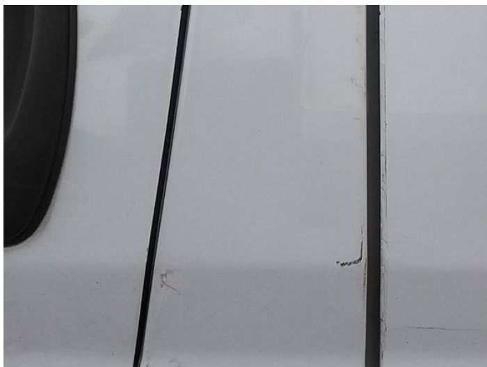
5: Panel Front Scratched Over 25mm Not Thru Paint
