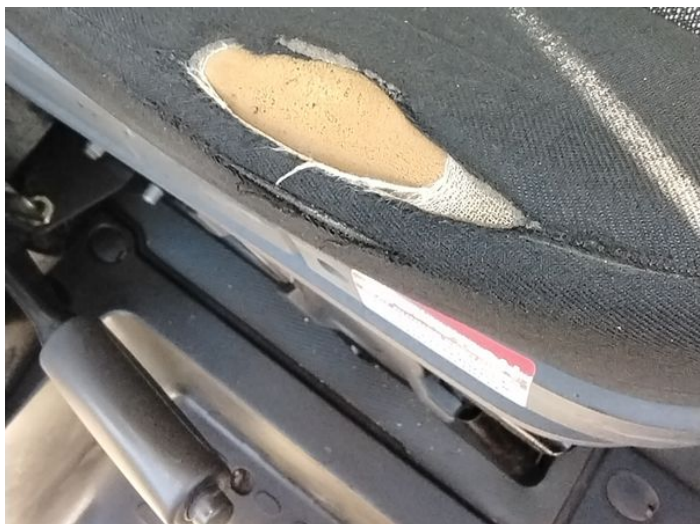
7: Seat Base Cover osf Torn Over 3mm
