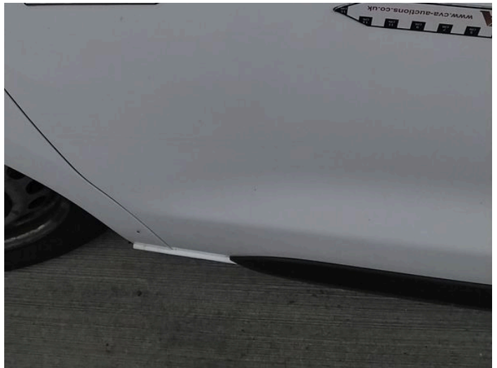
2: Door nsf Scratched Over 25mm Thru Paint
