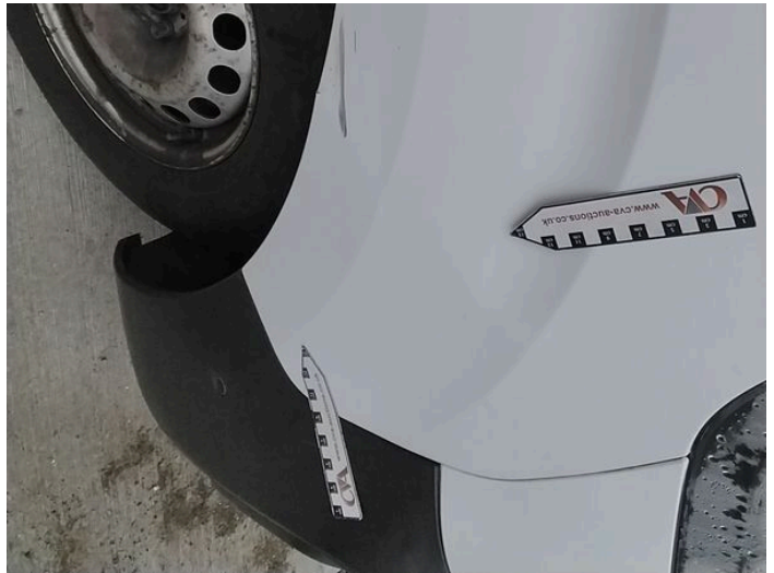
12: Wing osf Dented With Paint Damage
