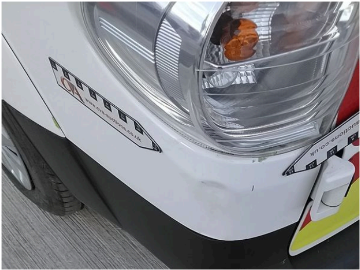
3: Qtr Panel nsr Dented Over 30mm
