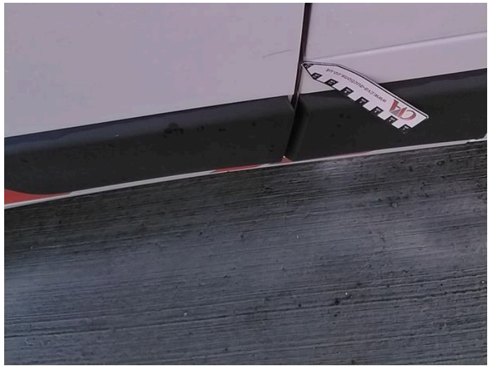
4: Door nsf Scratched Over 25mm Thru Paint
