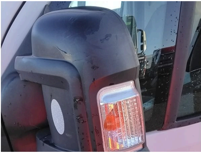
3: Door Mirror Assy nsf Broken Replace
