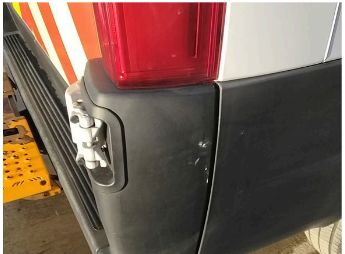
8: Bumper Rear Moulding Scuffed (Unpainted) UpTo 100mm
