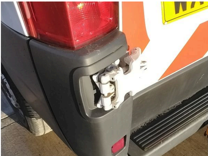
7: Bumper Rear Moulding Scuffed (Unpainted) UpTo 100mm
