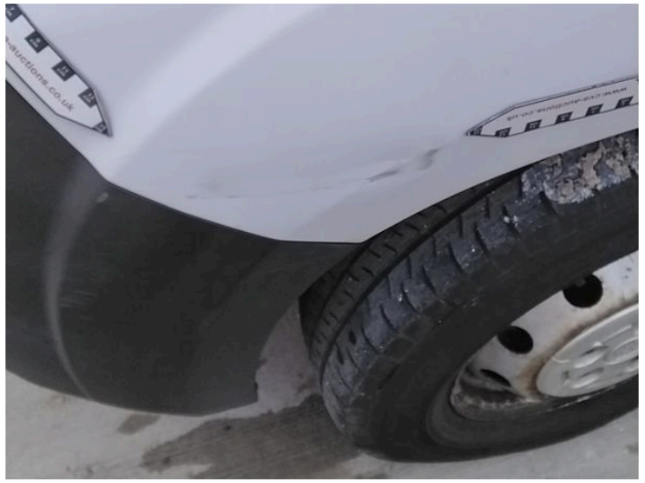
4: Wing nsf Dented With Paint Damage
