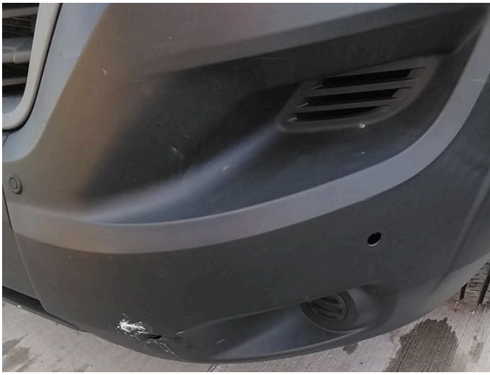
3: Bumper Front Moulding Broken Replace
