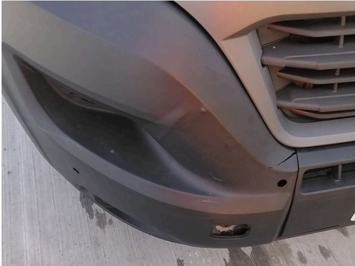
1: Bumper Front Moulding Broken Replace
