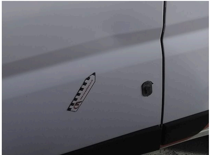
8: Qtr Panel nsr Dented Over 30mm
