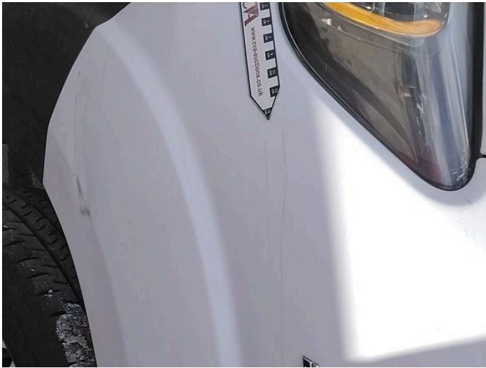
5: Wing nsf Scratched Over 25mm Thru Paint
