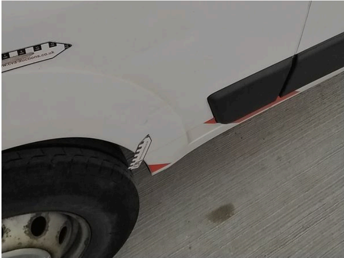
13: Qtr Panel osr Dented With Paint Damage
