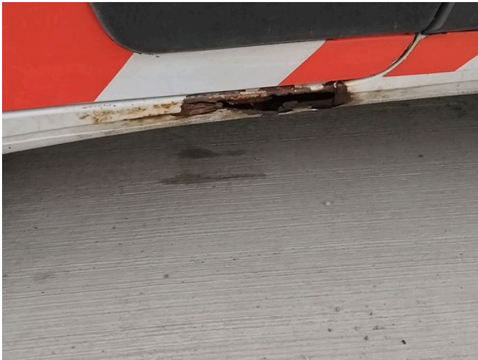
6: Sill ns Rusted Holed
