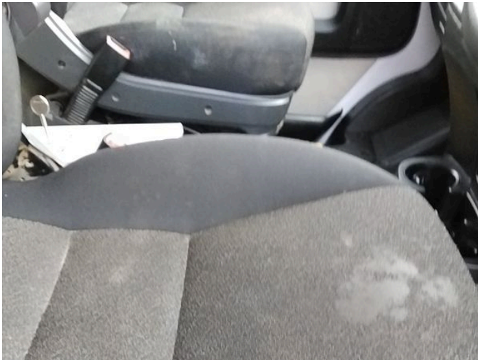
18: Seat Base Cover osf Torn Over 3mm
