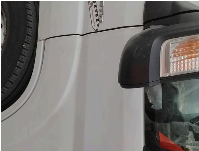
5: Door nsf Scratched Over 25mm Thru Paint
