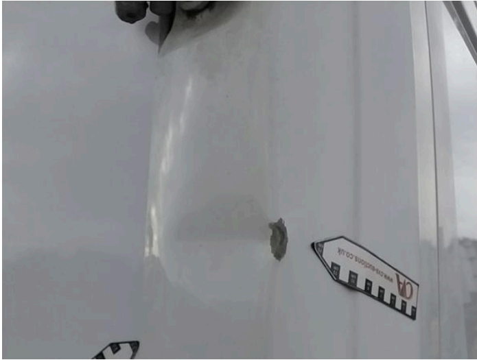
11: C Post os Dented With Paint Damage
