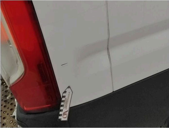
12: C Post os Dented With Paint Damage
