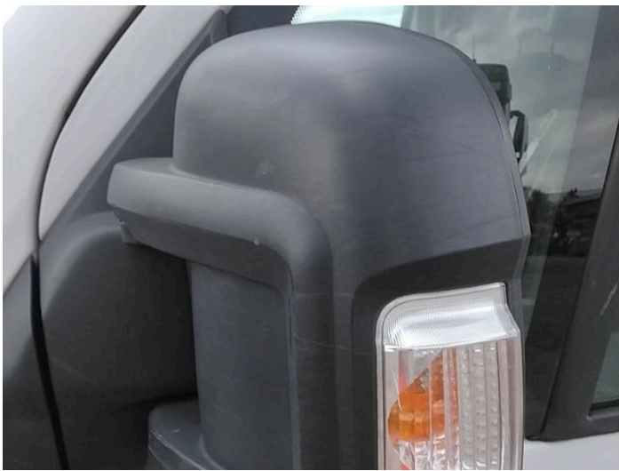
4: Door Mirror Assy nsf Broken Replace
