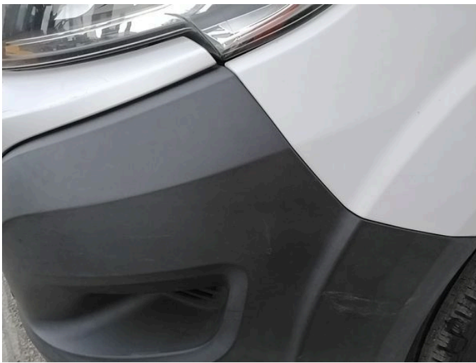
3: Bumper Front Moulding Scuffed (Unpainted) Over 100mm
