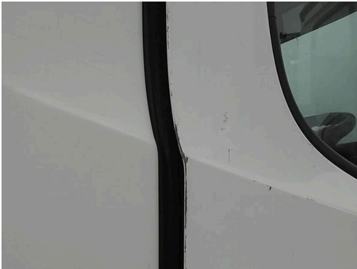
7: Door osf Chipped Edge Chip
