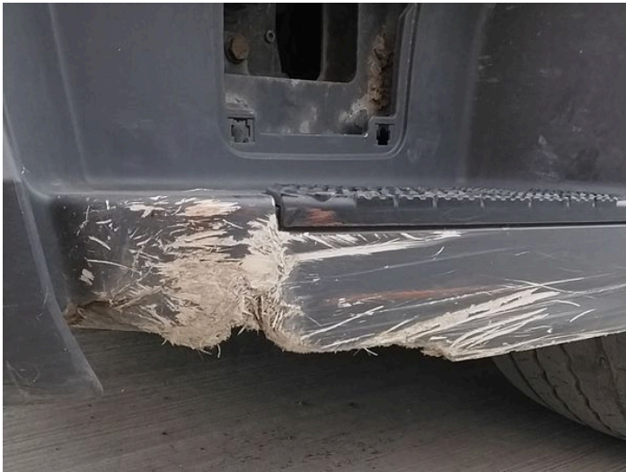
11: Moulding nsf Wing Broken Replace
