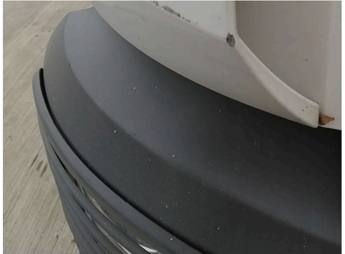
2: Panel Front Scratched Over 25mm Thru Paint
