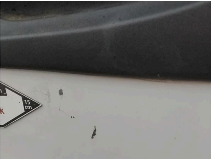
6: Door osf Scratched Over 25mm Thru Paint
