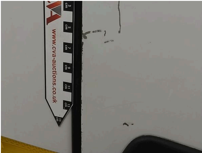
5: Door osf Scratched Over 25mm Thru Paint
