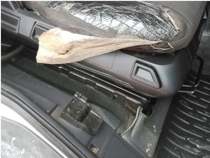
12: Seat Base Cover osf Torn Over 3mm
