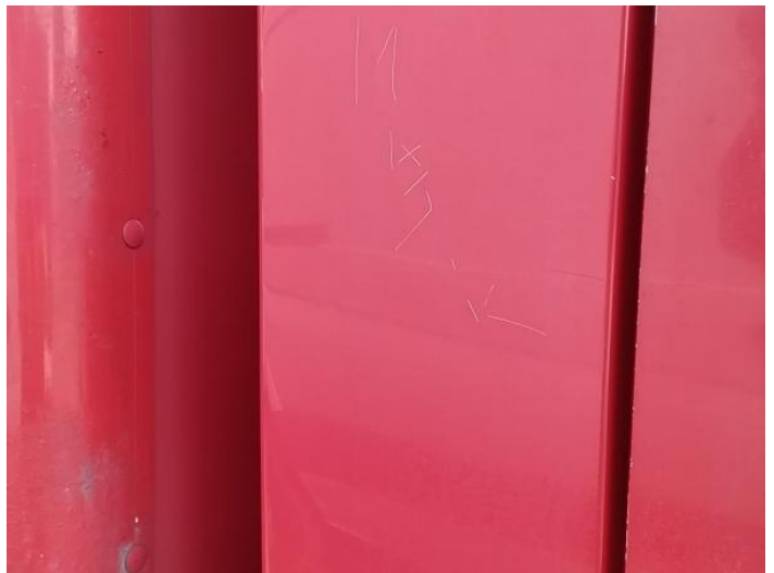
18: Door osf Scratched Over 25mm Thru Paint
