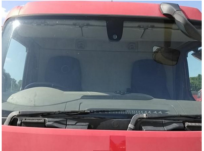
4: Screen Front Chipped Over 10mm
