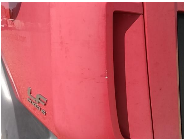
1: Moulding of Wing Scratched (Painted) Up To 25mm Thru Paint
