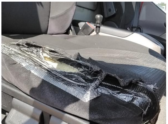
14: Seat Base Cover osf Torn Over 3mm
