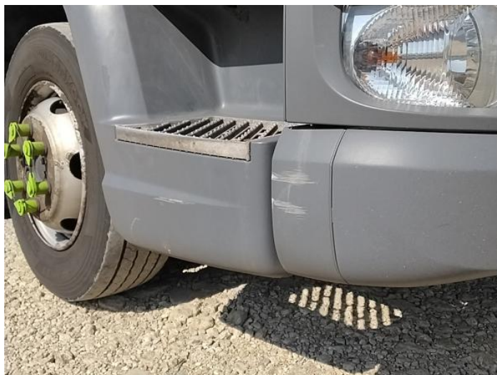
2: Bumper Front Scratched Over 100mm Thru Paint
