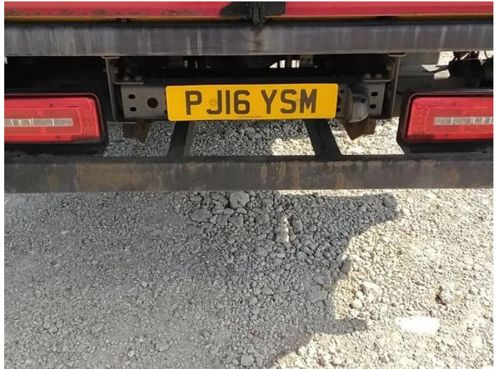
10: Bumper Rear Rusted Over 5mm
