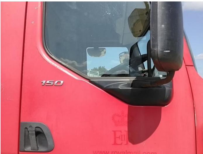
11: Door osf Scratched Over 25mm Thru Paint
