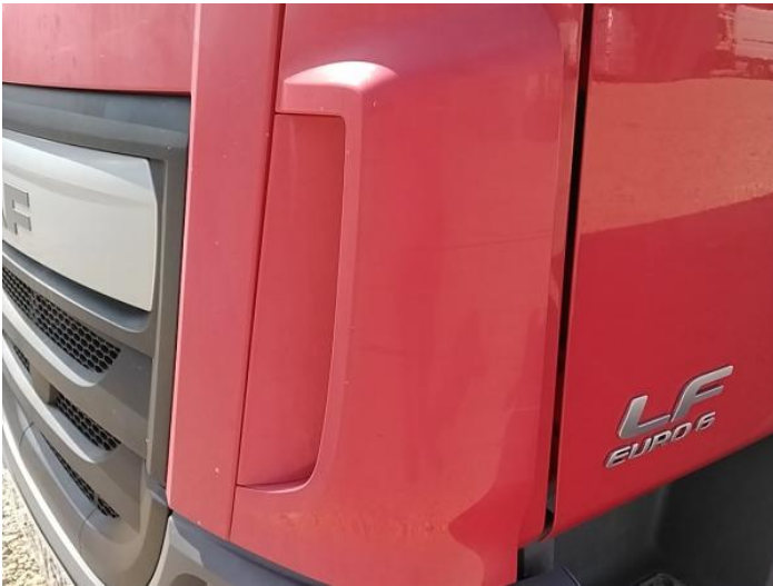
5: Moulding nsf Wing Scratched (Painted) Over 25mm Thru Paint
