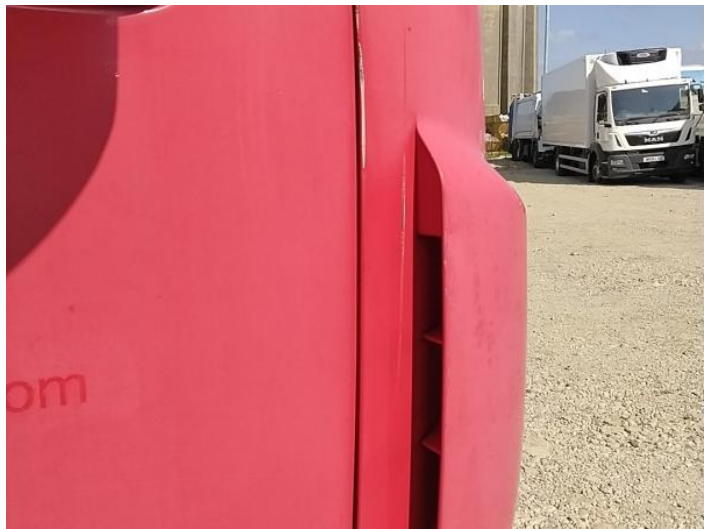
12: Moulding osf Wing Scratched (Painted) Over 25mm Thru Paint
