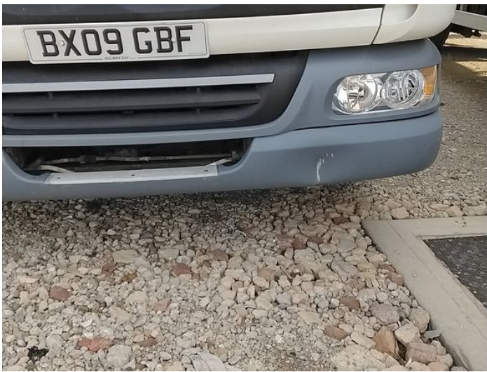
3: Bumper Front Dented With Paint Damage
