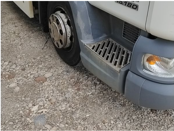
9: Wing Front Arch Extension os Scuffed (Unpainted) Over 100mm
