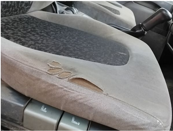
10: Seat Base Cover osf Holed Over 3mm
