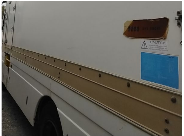
6: Qtr Panel nsr Scratched UpTo 25mm Not Thru Paint
