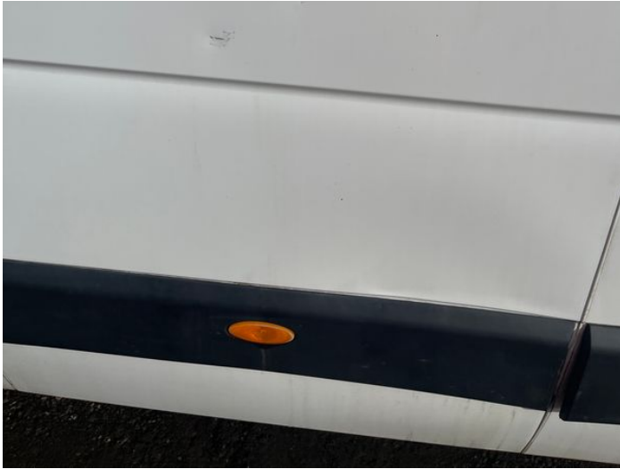
5: Qtr Panel osr Dented With Paint Damage
