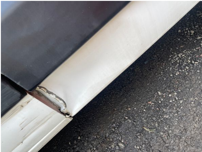
7: Qtr Panel osr Dented With Paint Damage
