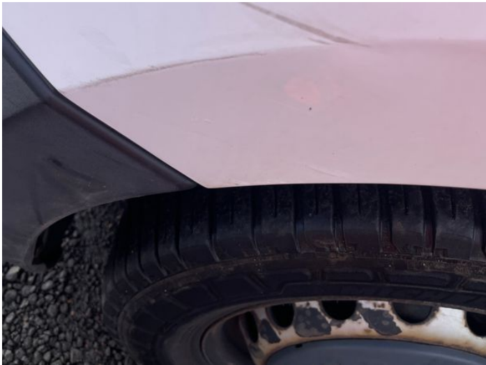
8: Panel Front Scratched Over 25mm Thru Paint
