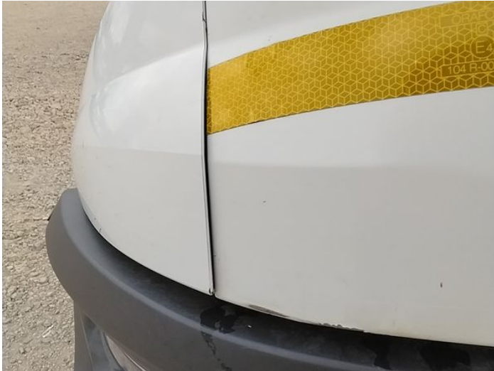
1: Panel Front Poor Previous Repair Poor Colour
