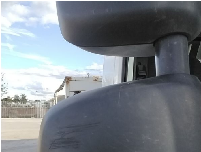
4: Door Moulding of Scuffed (Unpainted) Over 100mm
