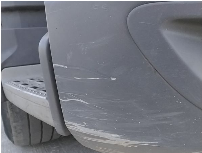
3: Bumper Front Moulding Scuffed (Unpainted) Over 100mm
