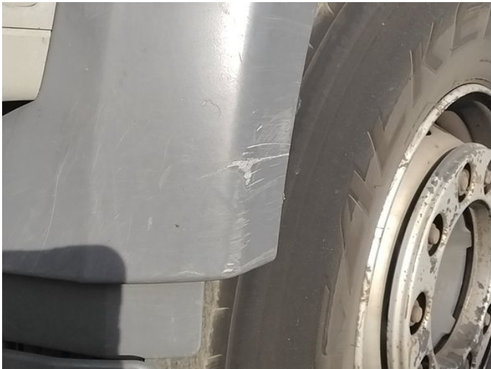
13: Moulding nsf Wing Scuffed (Unpainted) Over 100mm
