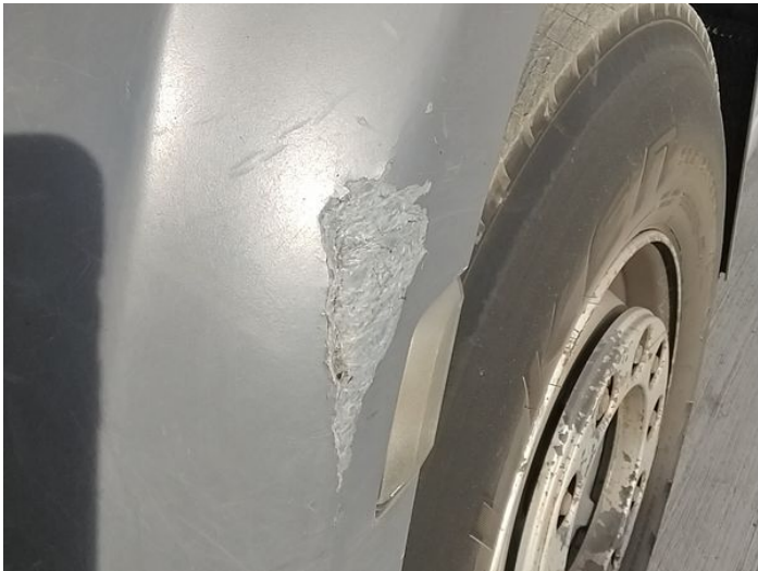
12: Moulding nsf Wing Broken Replace
