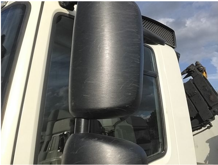
15: Door Mirror Assy nsf Scuffed (Unpainted) Over 100mm
