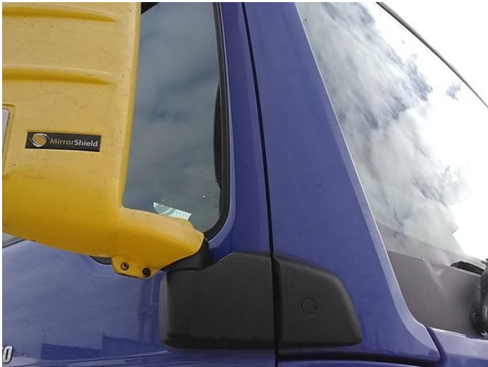
14: A Post os Scratched Over 25mm Not Thru Paint
