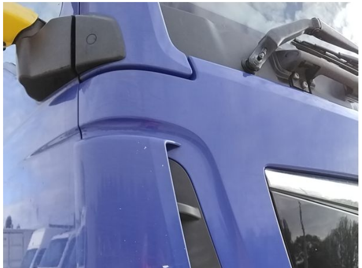
2: Wing and Chipped Multiple Chips
