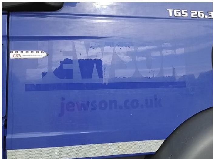
8: Door nsf Scratched Over 25mm Not Thru Paint
