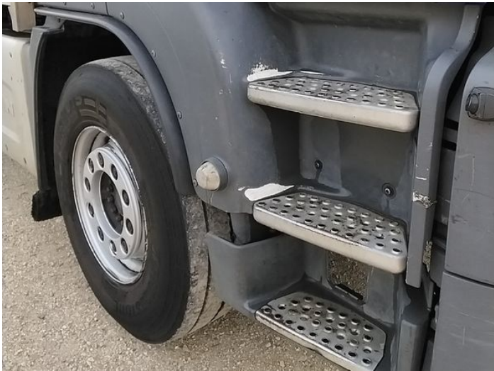
13: Wing Front Arch Extension os Scuffed (Unpainted) Over 100mm
