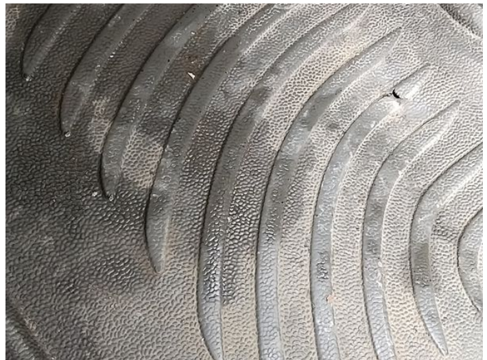
18: Carpets Front Holed Over 3mm
