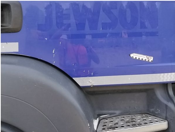
12: Door osf Scratched Over 25mm Thru Paint
