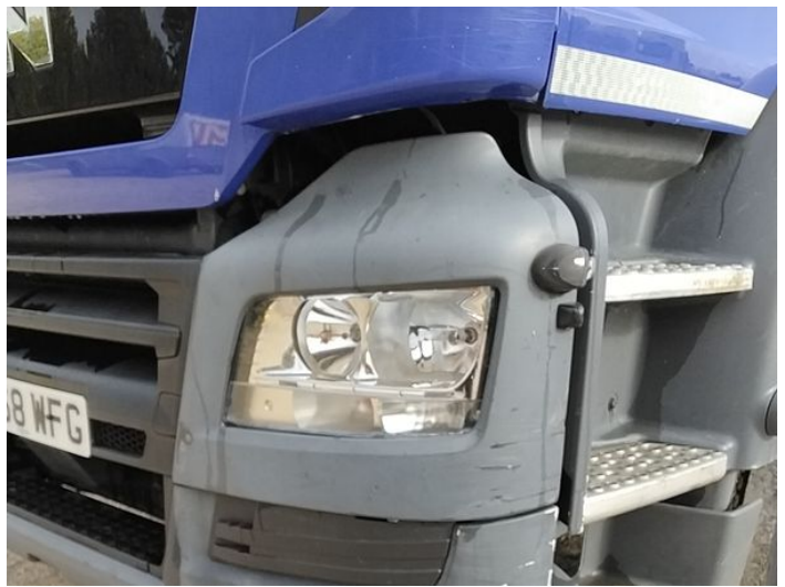
4: Bumper Front Moulding Scuffed (Unpainted) Over 100mm
