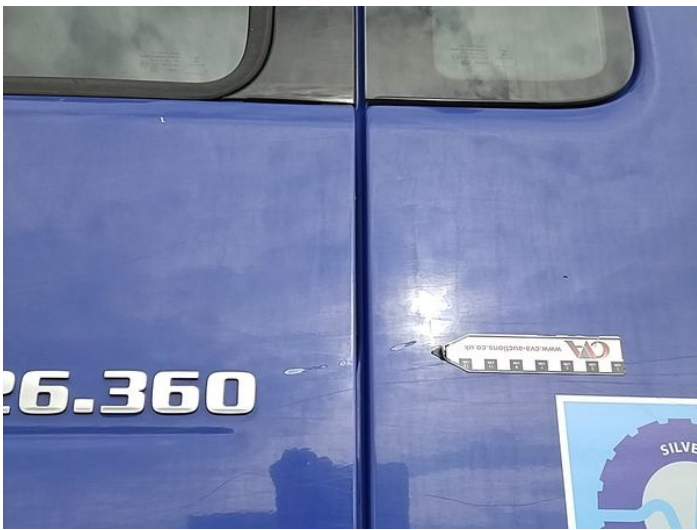
9: Door nsf Scratched UpTo 25mm Thru Paint
