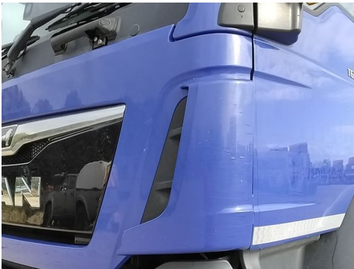
5: Wing nsf Scratched Over 25mm Not Thru Paint
