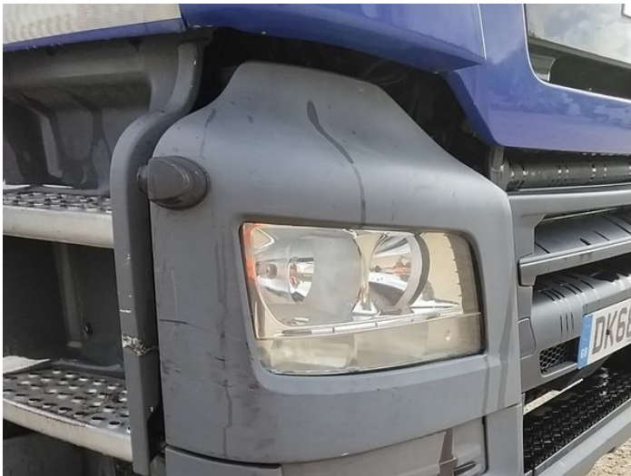
1: Bumper Front Moulding Scuffed (Unpainted) Over 100mm
