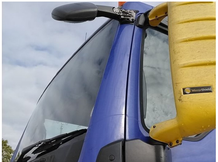
6: A Post ns Scratched Over 25mm Not Thru Paint
